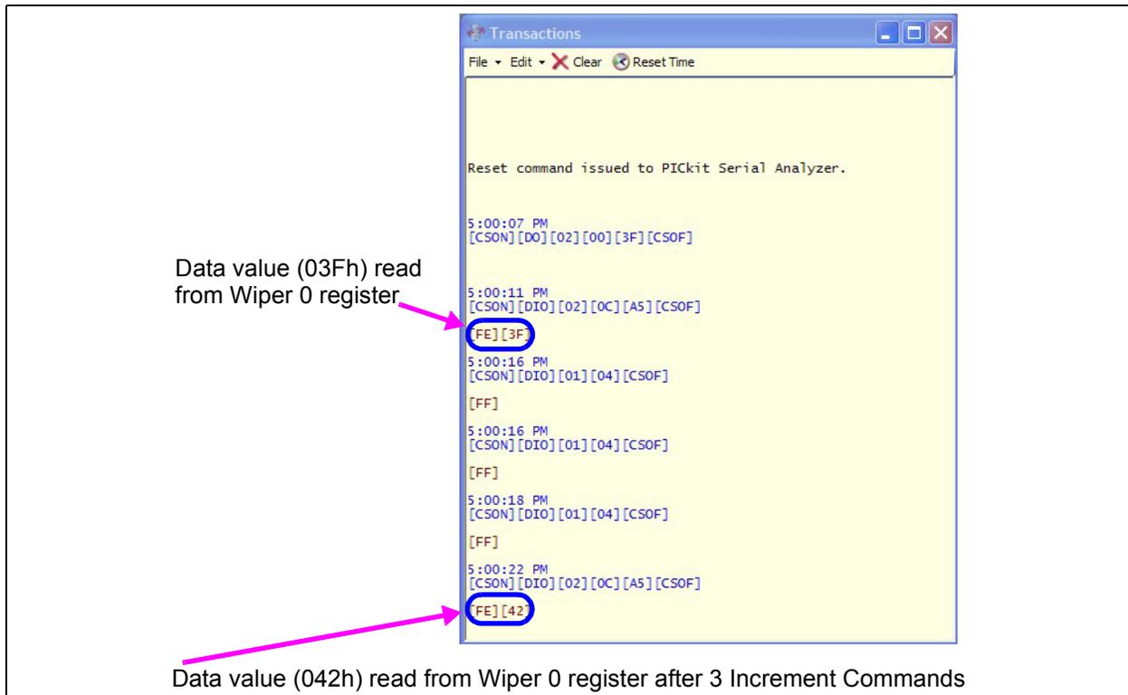
**FIGURE 2-15:** MCP4261 Transaction Window – Wiper 0 Increments.
