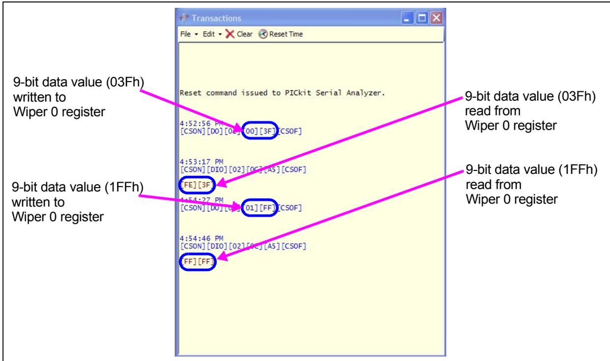
**FIGURE 2-13:** MCP4261 Transaction Window – Wiper 0 Writes and Reads.
