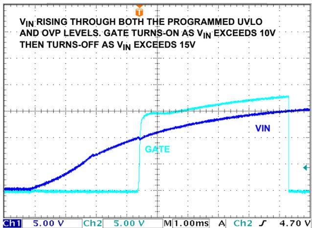
FIGURE 31. ISL6146C RISING V<sub>IN</sub>, UVLO AND OVP FUNCTION
