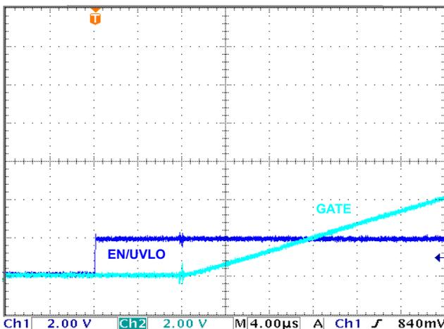
FIGURE 25. ISL6146A/D EN/ISL6146C UVLO TO GATE ON DELAY
