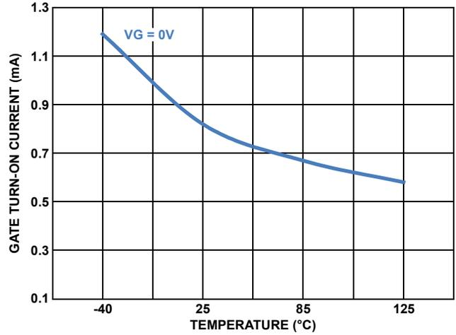
FIGURE 10. GATE TURN-ON CURRENT  $V_{IN} = 12V$
