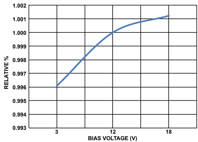
FIGURE 18. EN/EN/OVP/UVLO V<sub>th</sub> DELTA vs BIAS VOLTAGE NORMALIZED TO BIAS = 12V
