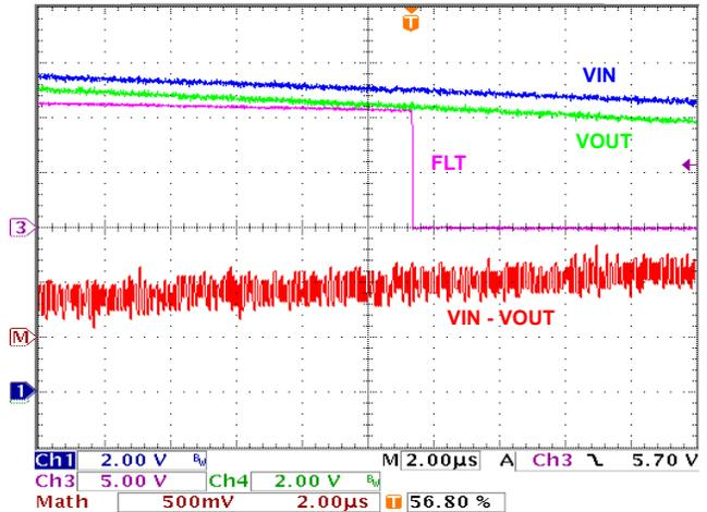
FIGURE 40. FAULT ASSERTING  $V_{IN}$  TO  $V_{OUT} > V_{FWD\_FLT}$
