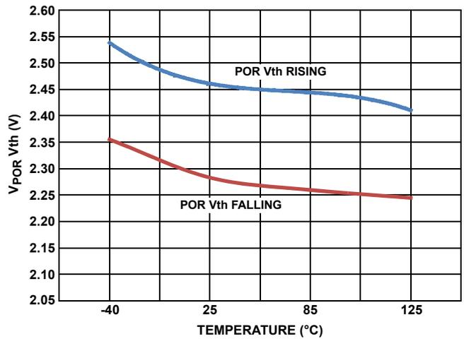
FIGURE 6. POR  $V_{th}$  RISING AND FALLING VOLTAGE
