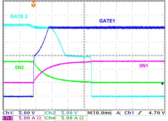
FIGURE 22. ISL6146C SLOW RAMP DISCONNECT 12V OR-ing
