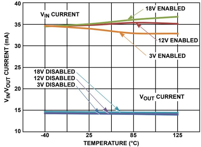
FIGURE 4. ISL6146A/B/C/D/E  $V_{IN}$  AND  $V_{OUT}$  CURRENT vs TEMPERATURE
