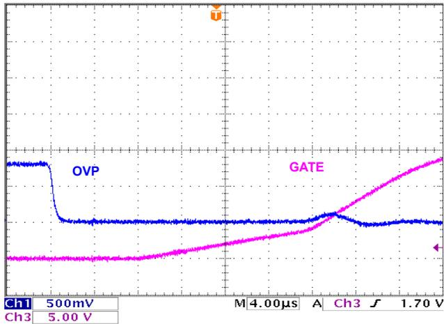
FIGURE 29. ISL6146C OVP TO GATE ON DELAY
