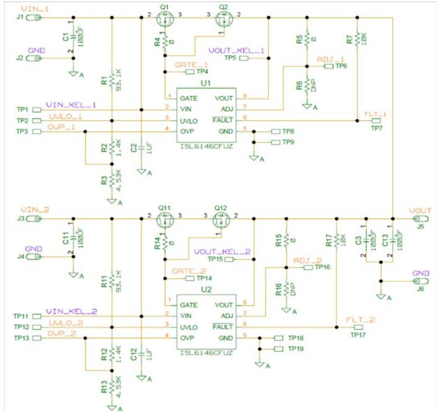
FIGURE 61. ISL6146CEVAL1Z SCHEMATIC
