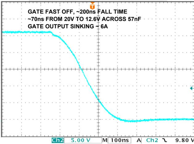
FIGURE 35. FAST GATE TURN-OFF WITH 57nF GATE
