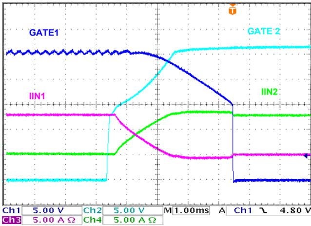
FIGURE 21. ISL6146C SLOW RAMP CONNECT 12V OR-ing
