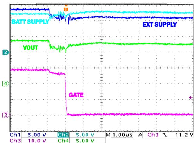
FIGURE 55. EXTERNAL SUPPLY > BATT SUPPLY DISCONNECTED
