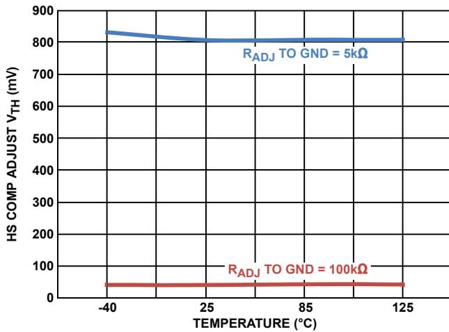
FIGURE 17. HS COMPARATOR ADJUSTABLE V<sub>th</sub>
