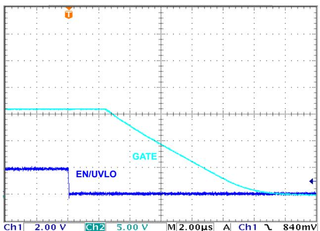
FIGURE 26. ISL6146A/D EN/ISL6146C UVLO TO GATE OFF DELAY
