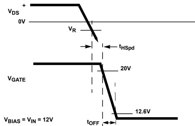
FIGURE 44. FAST RAMP REVERSE PROTECTION TIMING DIAGRAM
