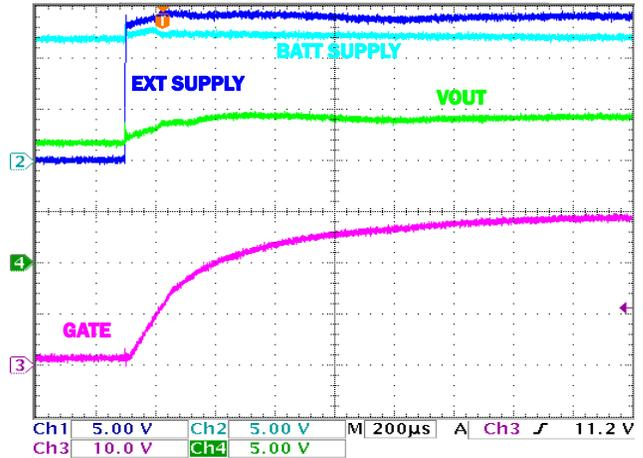
FIGURE 54. EXTERNAL SUPPLY > BATT SUPPLY CONNECTED
