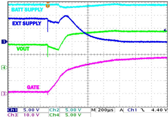
FIGURE 52. EXTERNAL SUPPLY < BATT SUPPLY DISCONNECTED
