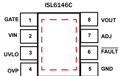
EPAD on DFN only, connect to GND
