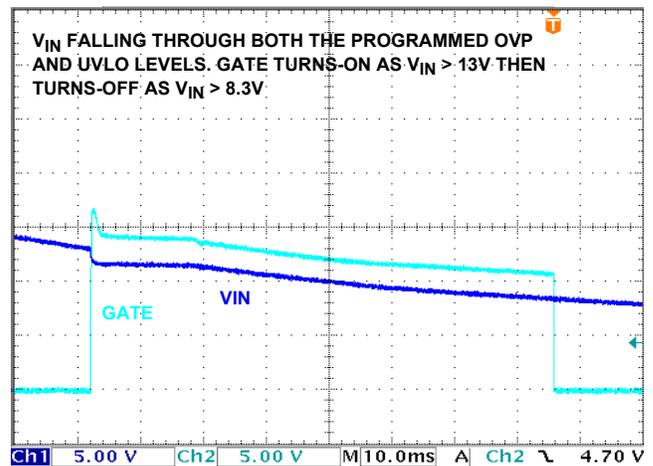
FIGURE 32. ISL6146C FALLING, V<sub>IN</sub> OVP AND UVLO FUNCTION
