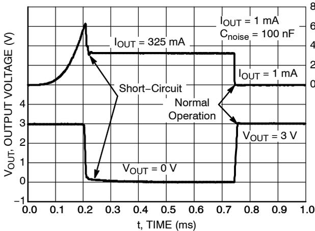
**Figure 41. Short-Circuit Protection**,
