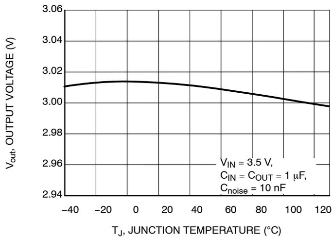
**Figure 5. Output Voltage vs. Junction Temperature,  $V_{OUT} = 3.0$  V**
