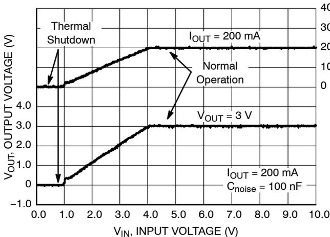
**Figure 43. Thermal Shutdown Protection**
