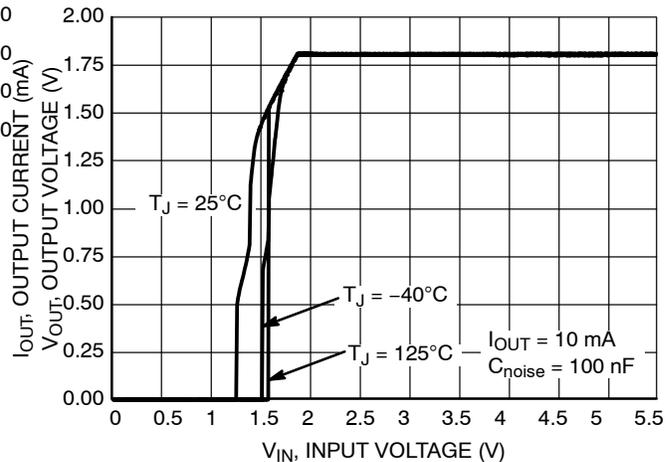
**Figure 44. Output Voltage vs. Input Voltage**,
