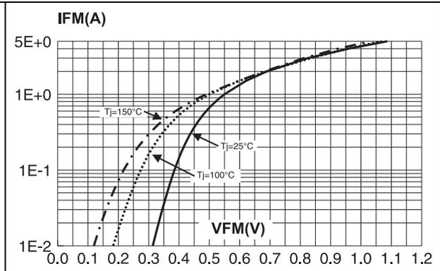
**Figure 9. Forward voltage drop versus forward current (low level, maximum values)**
