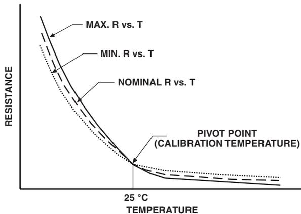
Point match resistance tolerances at temperatures other than 25 °C are not the same as the calibration temperature. This difference is presented in Figure 2.
