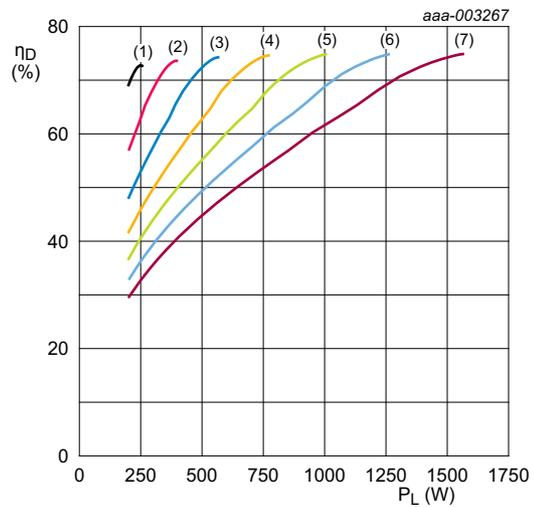
$I_{Dq} = 40 \text{ mA}$ ;  $f = 108 \text{ MHz}$ ;  $t_p = 100 \text{ }\mu\text{s}$ ;  $\delta = 20 \text{ \%}$ .
