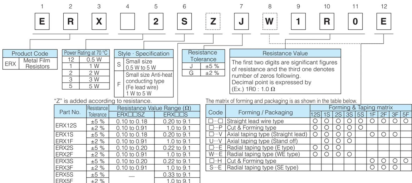
The above example 1 shows a small metal film resistor, 2 W power rating, resistance value of 1.0 Ω, tolerance ±5 %, and package of radial taping.
