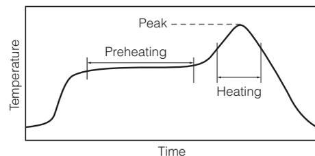
For soldering (Example : Sn/Pb)
