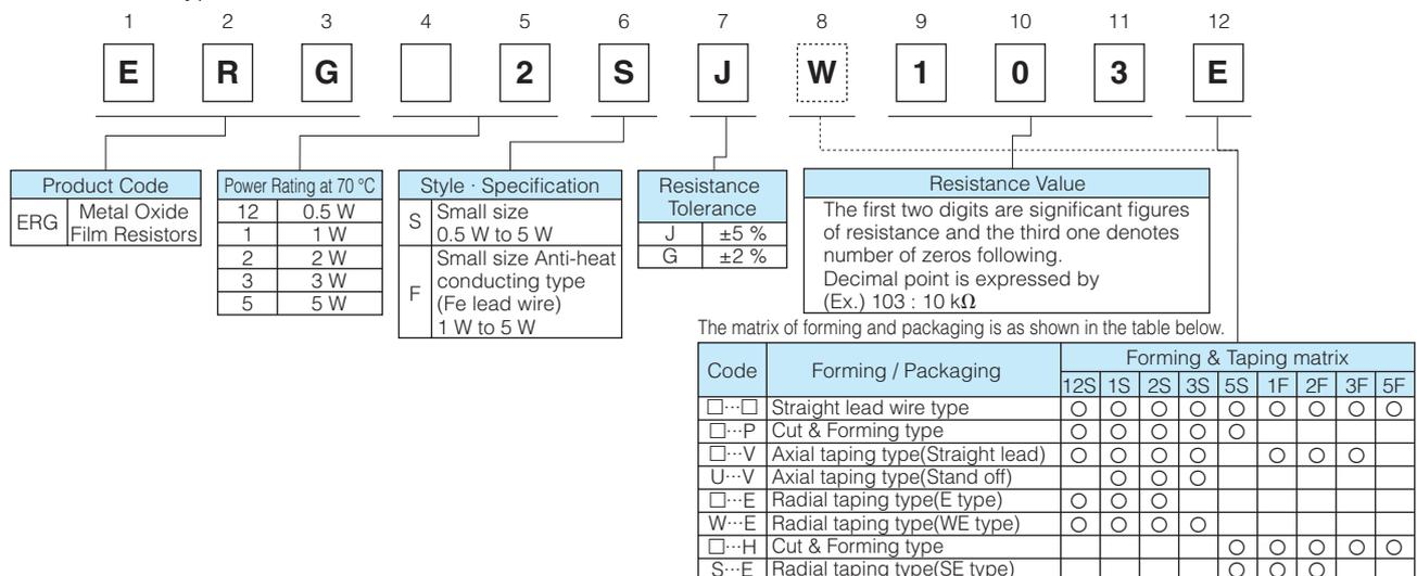
The above example 2 shows a small metal oxide film resistor, 2 W power rating, resistance value of 10 kΩ, tolerance ±5 %, and package of radial taping.
