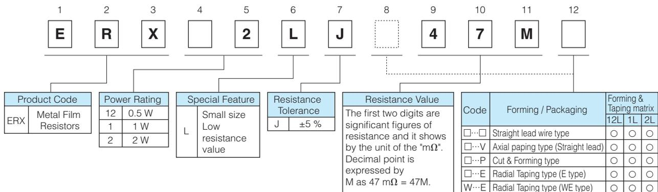
The above example shows a small size and low resistance value metal film resistor, 2 W power rating, resistance value of 47 m ohms, tolerance ±5 %, and package of standard bulk packing.
