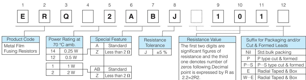
The above example shows a standard Metal Film Fusing Resistors, 2 W power rating, resistance value of 100 Ω, tolerance of ±5 %, and package of standard bulk packing.
