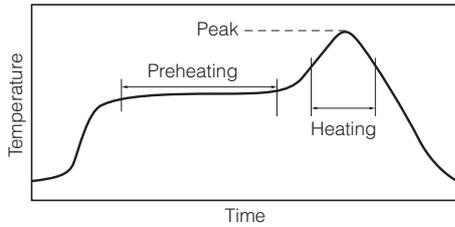
For soldering (Example : Sn/Pb)
