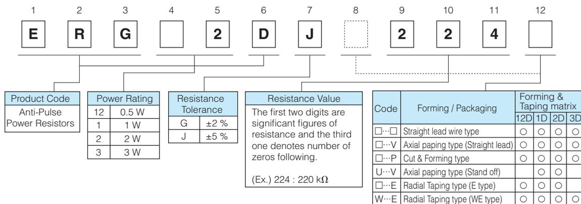
The above example shows an anti-pulse resistor, 2 W power rating, resistance value of 220 k ohms, tolerance ±5 %, and package of standard bulk packing.
