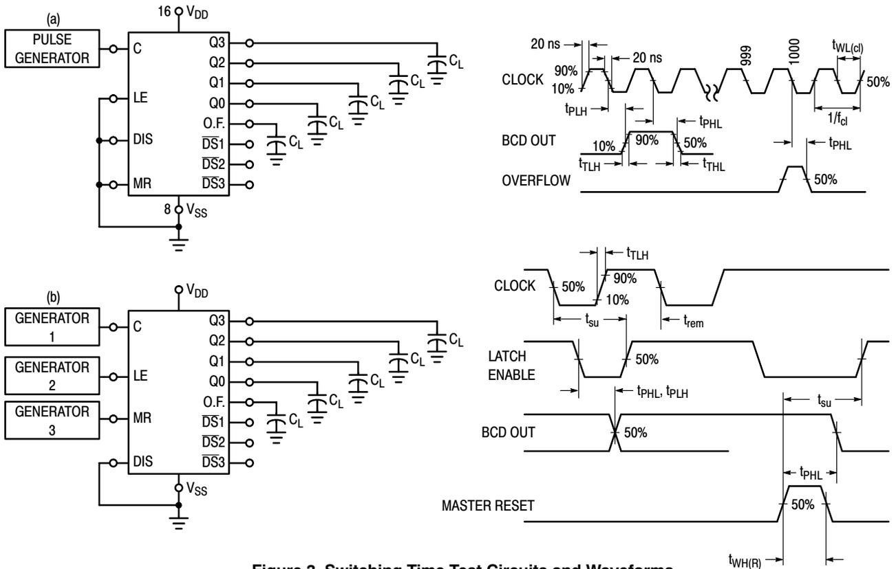
Figure 3. Switching Time Test Circuits and Waveforms
