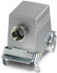
HEAVYCON sleeve housing D50, with double locking latch, height 76 mm, with support 1x M32, lateral conductor exit
