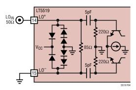
Figure 4. LO Input Circuit
