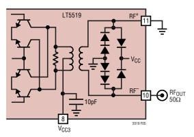
Figure 5. RF Output Circuit
