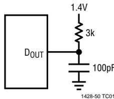
Load Circuit for t<sub>DZ</sub>, t<sub>DV</sub>
