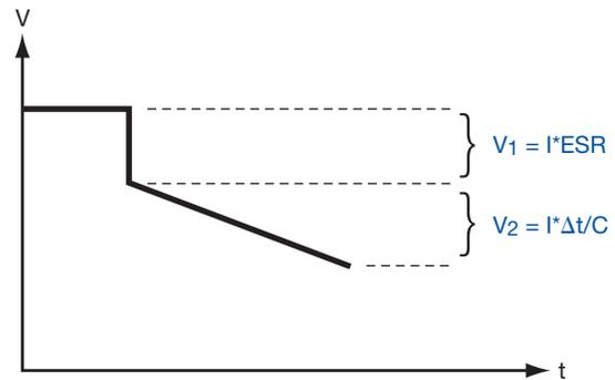
It is assumed that during the pulse, 0.5A is delivered by the battery and 1.5A by the capacitor.
