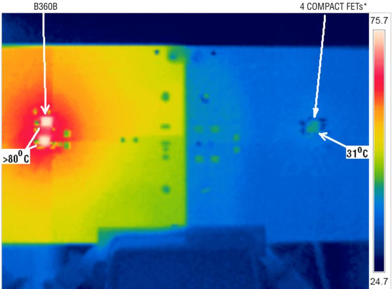
CONDITION: 13VDC<sub>IN</sub>, 3A LOAD ON SAME PCB
