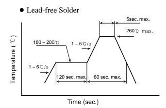
**Note:** Number of reflow process shall be less than 2 times and cooling process to normal temperature is required between first and Second soldering process.
