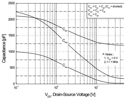
Figure 5. Capacitance Characteristics
