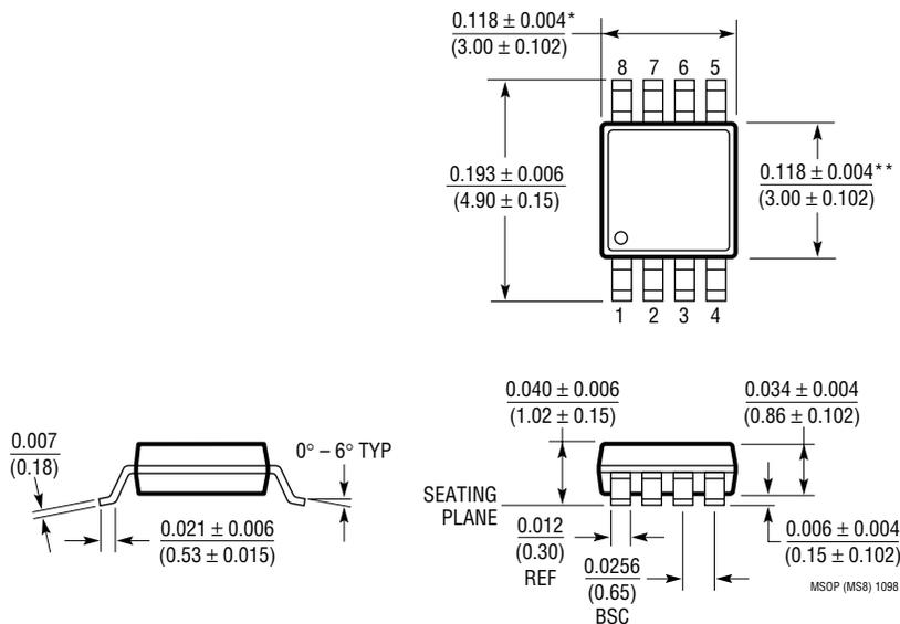
\* DIMENSION DOES NOT INCLUDE MOLD FLASH, PROTRUSIONS OR GATE BURRS. MOLD FLASH, PROTRUSIONS OR GATE BURRS SHALL NOT EXCEED 0.006" (0.152mm) PER SIDE
