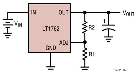
$$V_{\text{OUT}} = 1.22\text{V} \left( 1 + \frac{R_2}{R_1} \right) + (I_{\text{ADJ}})(R_2)$$
