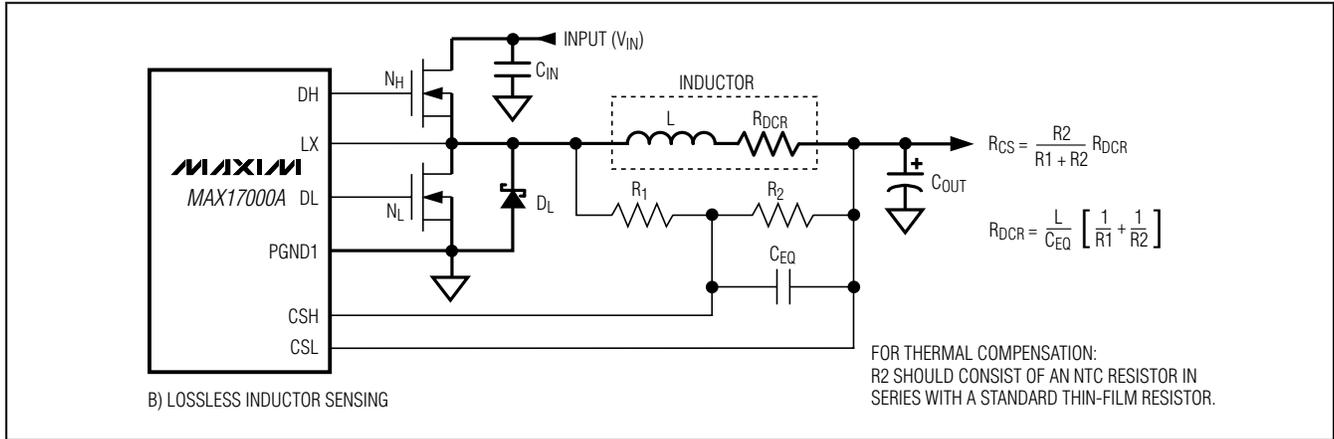
Figure 7b. Current-Sense Configurations (Sheet 2 of 2)
