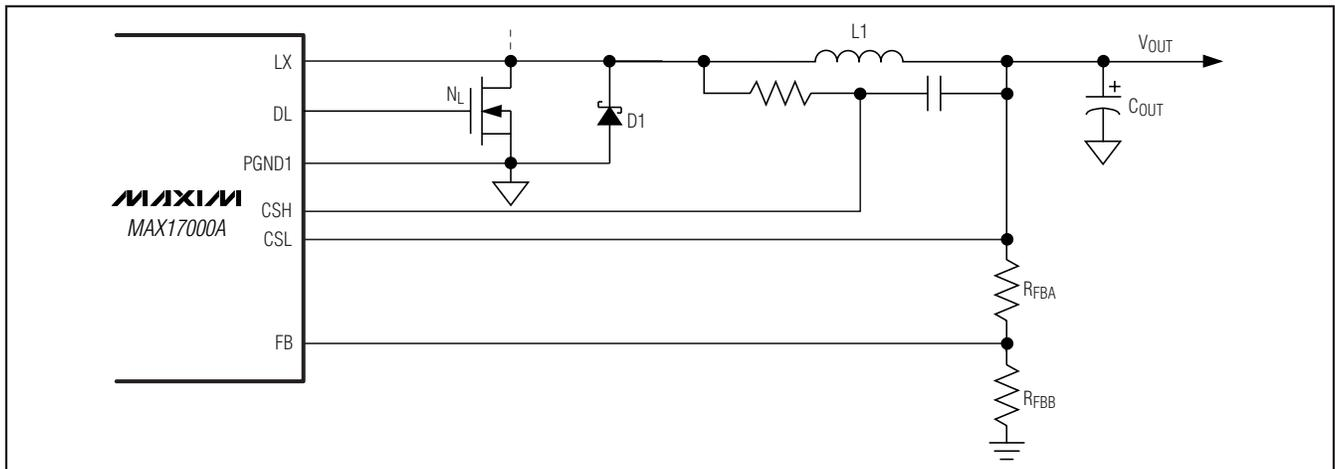
Figure 8. Setting  $V_{OUT}$  with a Resistive Voltage-Divider
