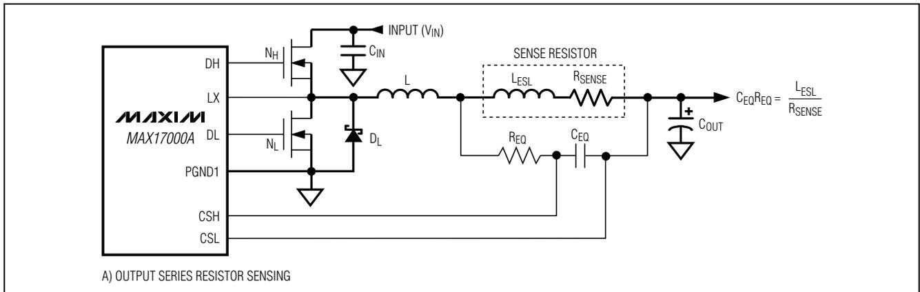
Figure 7a. Current-Sense Configurations (Sheet 1 of 2)
