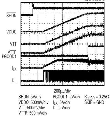
**SHUTDOWN WAVEFORM (DISCHARGE MODE ENABLED)**
