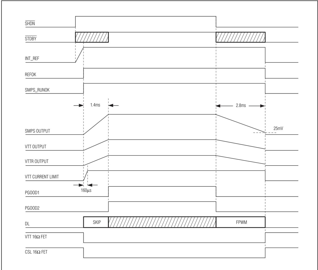
Figure 6. MAX17000A Startup/Shutdown Timing with OVP Enabled
