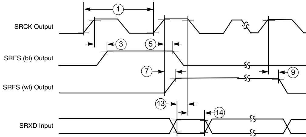
Figure 60. SSI Receiver Internal Clock Timing Diagram
