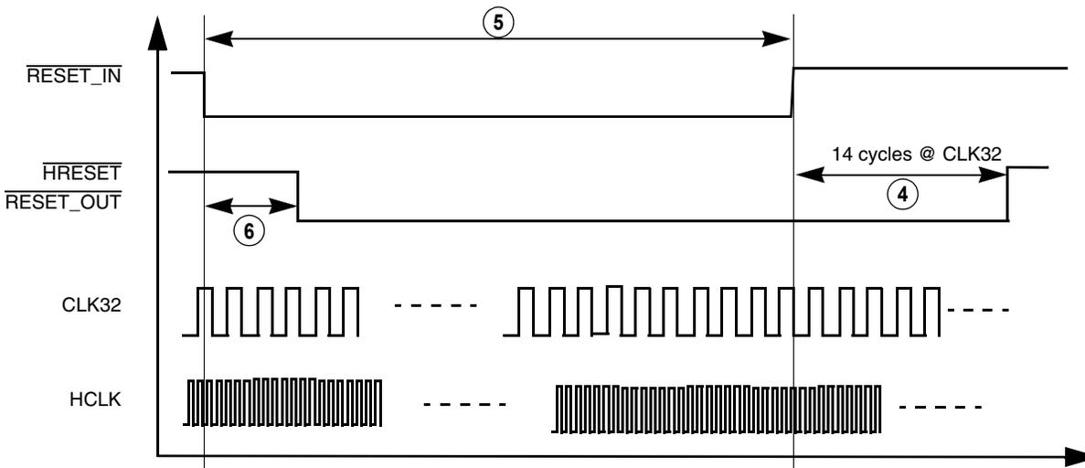
Figure 4. Timing Relationship with RESET\_IN
