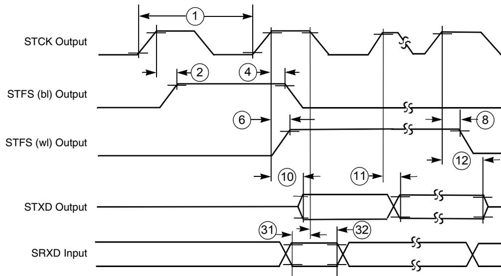
**Note:** SRXD input in synchronous mode only.
