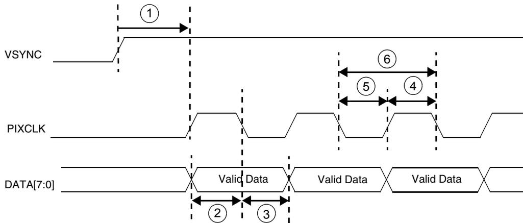
**Figure 66. Sensor Output Data on Pixel Clock Rising Edge
