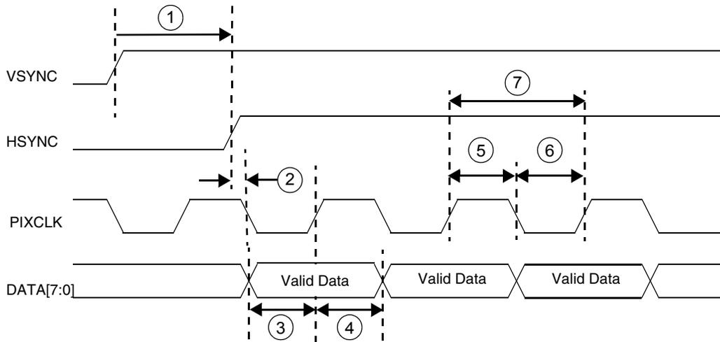
**Figure 63. Sensor Output Data on Pixel Clock Falling Edge
