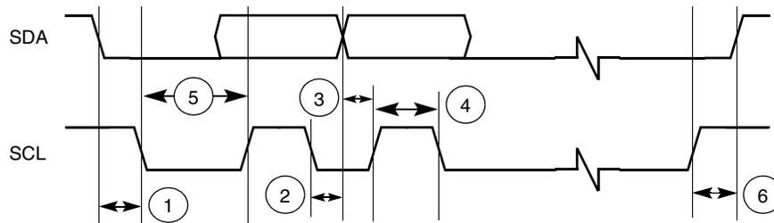
Figure 58. Definition of Bus Timing for I<sup>2</sup>C
