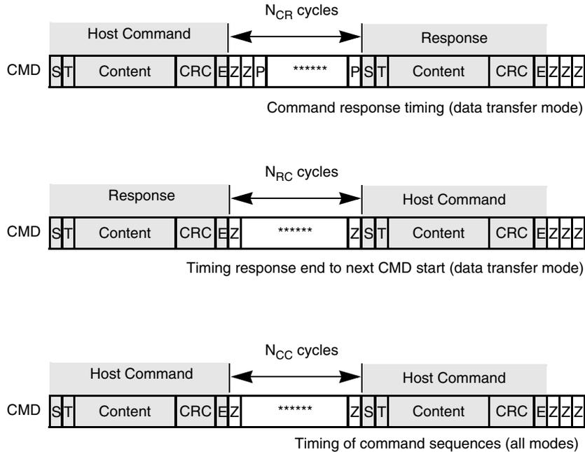
Figure 44. Timing Diagrams at Data Transfer Mode
