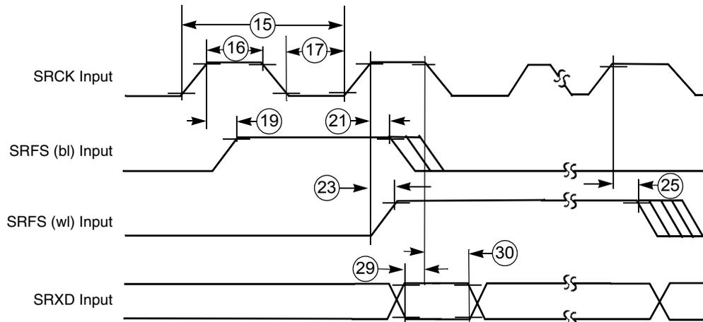
Figure 62. SSI Receiver External Clock Timing Diagram
