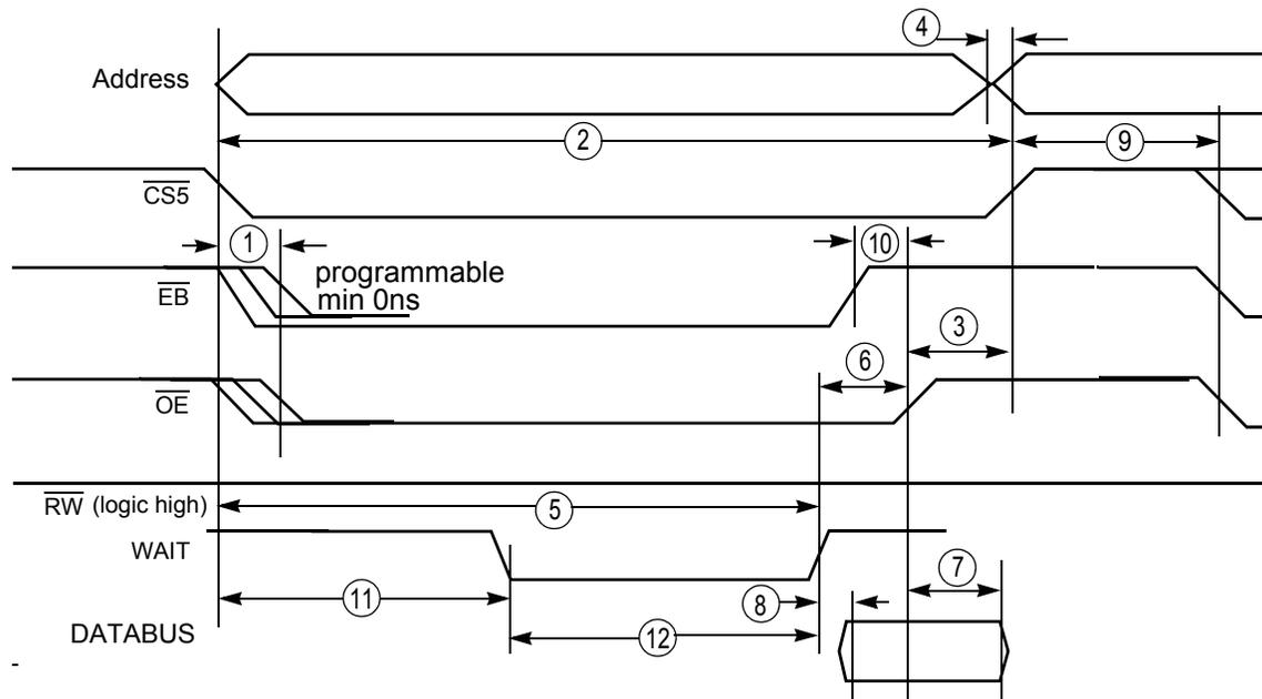
Figure 7. DTACK WAIT Read Cycle DMA Enabled
