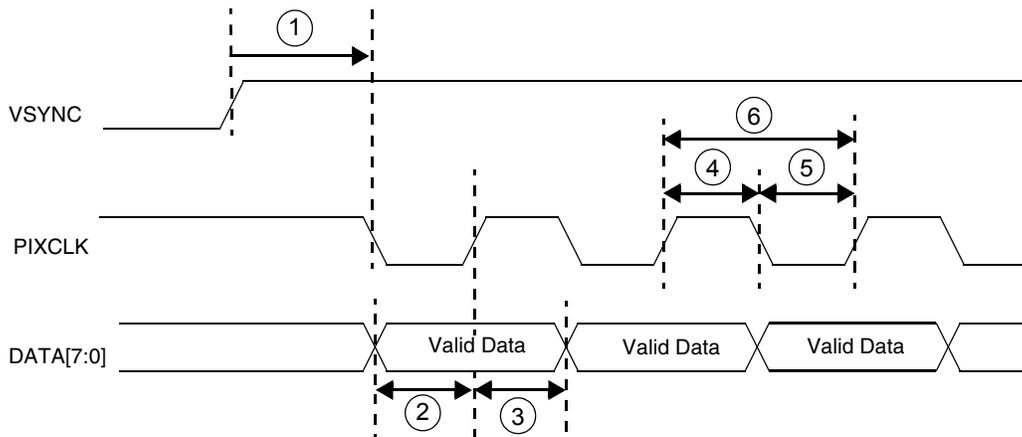
Figure 65. Sensor Output Data on Pixel Clock Falling Edge
