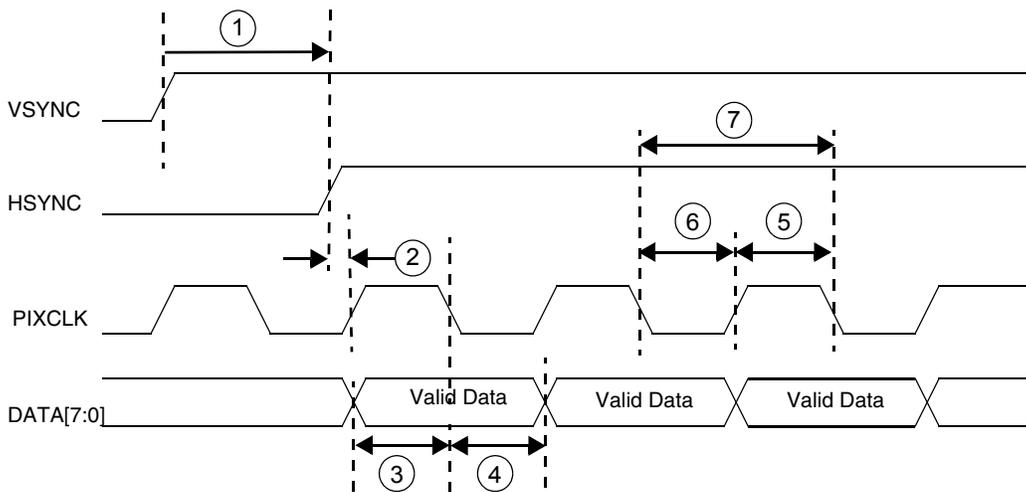
**Figure 64. Sensor Output Data on Pixel Clock Rising Edge
