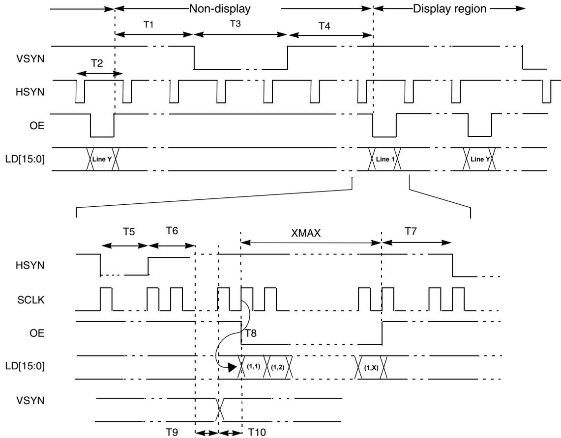
**Figure 41. 4/8/16 Bit/Pixel TFT Color Mode Panel Timing**
