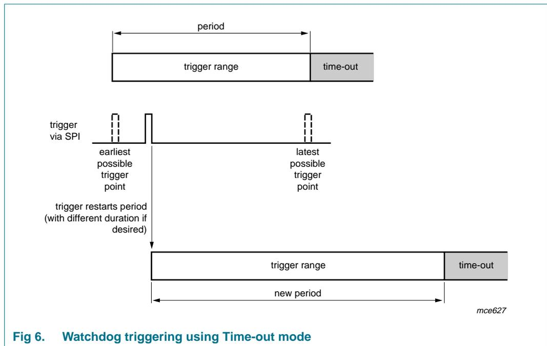
Fig 6. Watchdog triggering using Time-out mode
