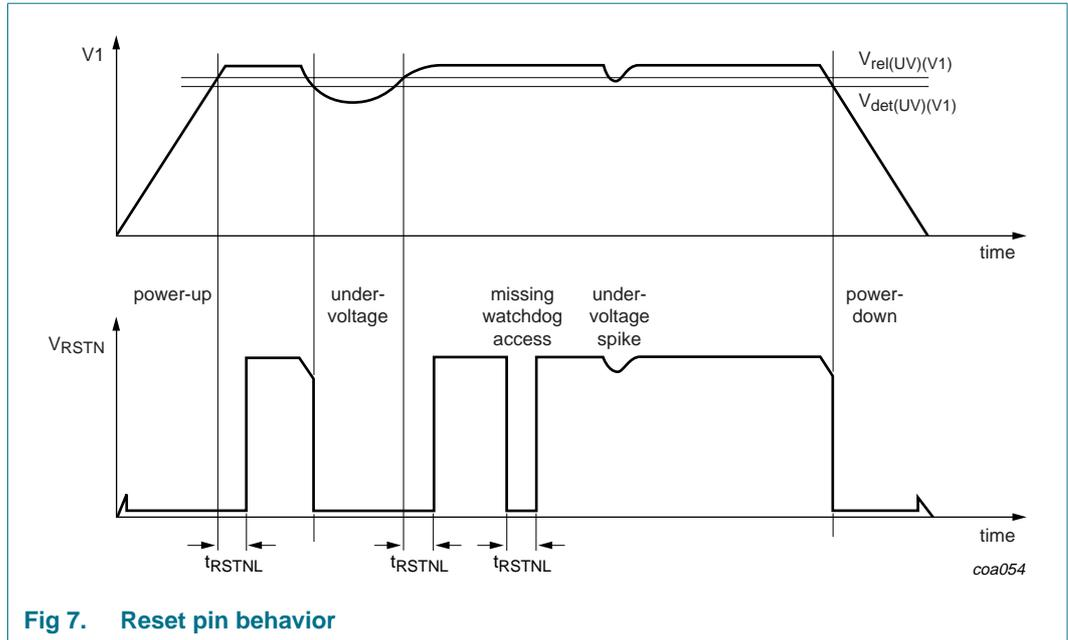
Fig 7. Reset pin behavior
