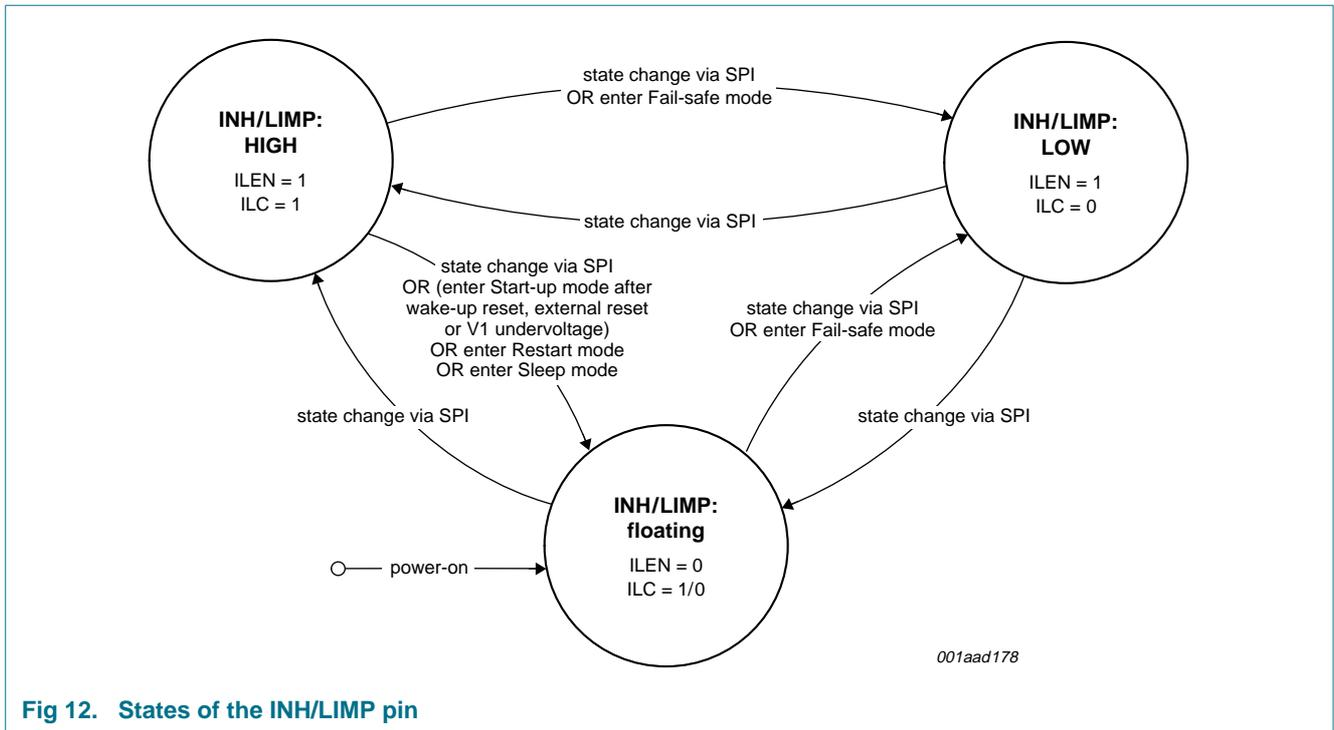
Fig 12. States of the INH/LIMP pin
