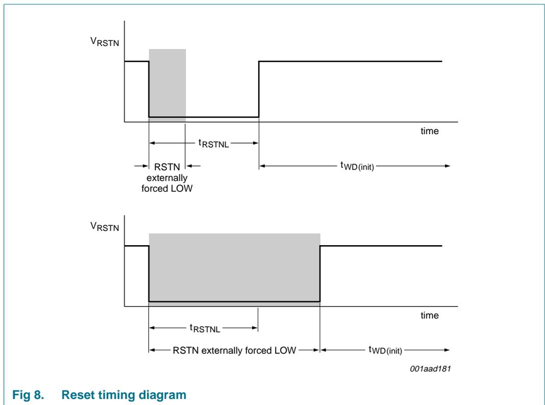
Fig 8. Reset timing diagram
