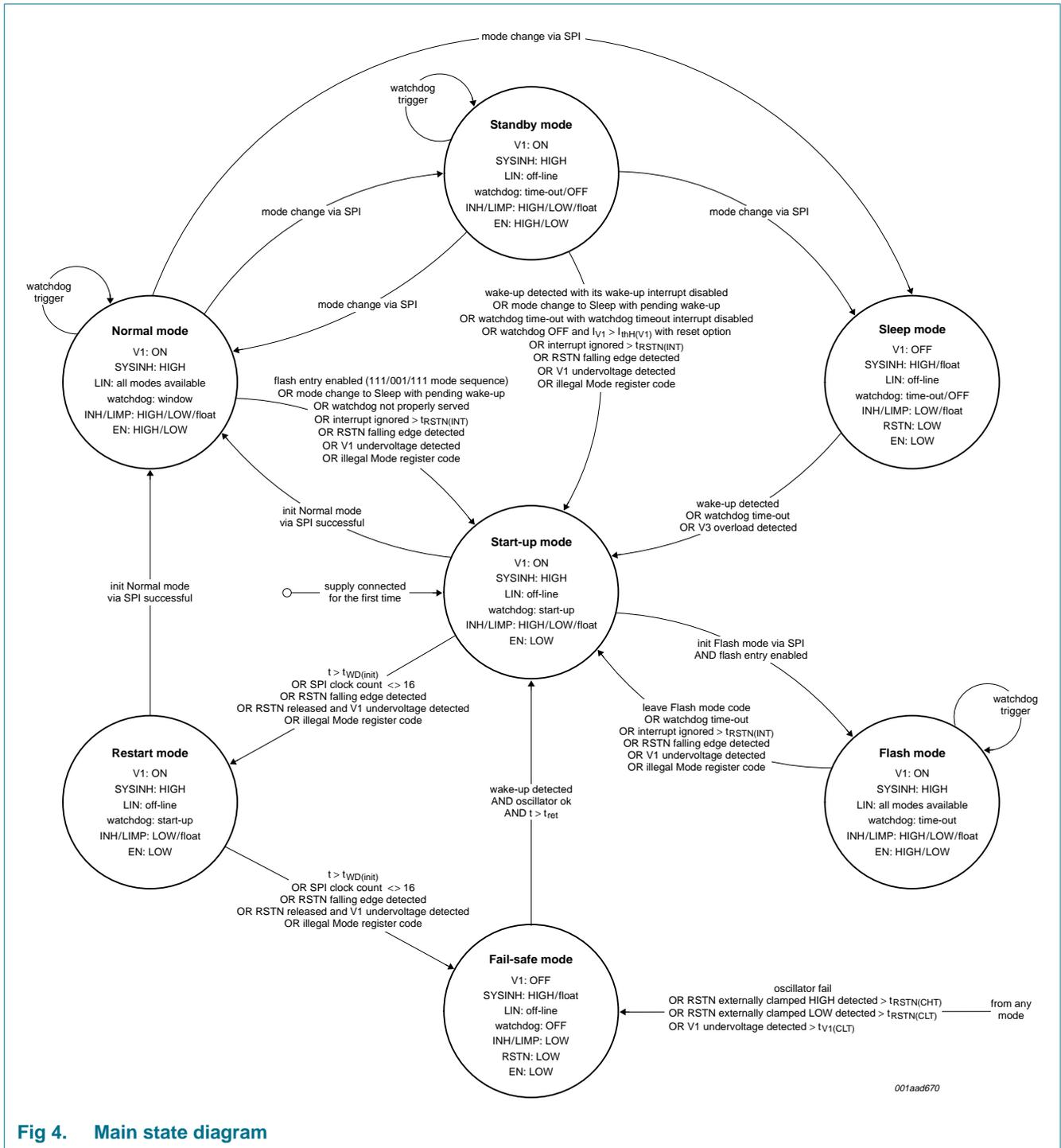
Fig 4. Main state diagram
