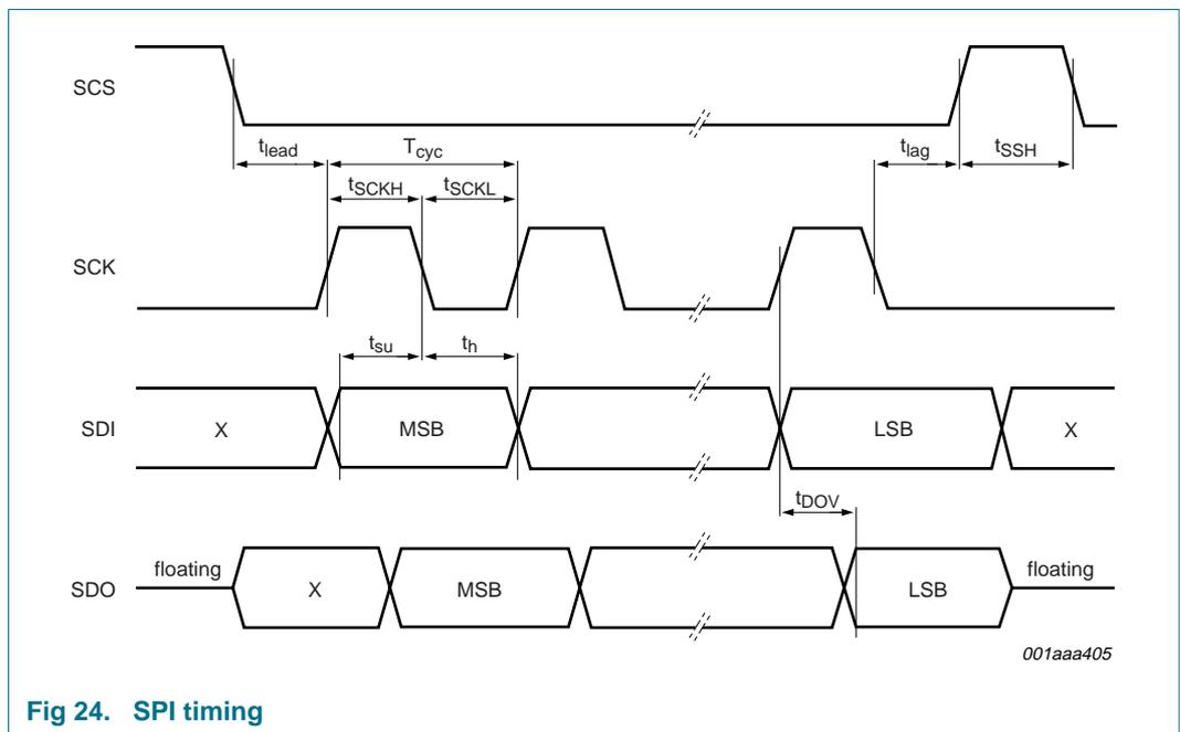
**Fig 24. SPI timing**
