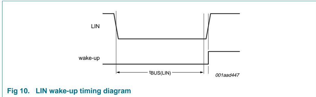
Fig 10. LIN wake-up timing diagram
