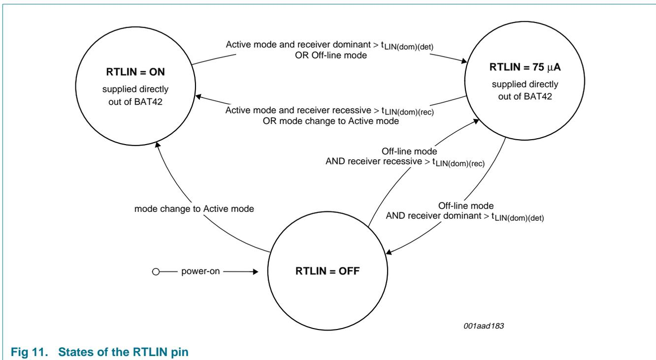
Fig 11. States of the RTLIN pin
