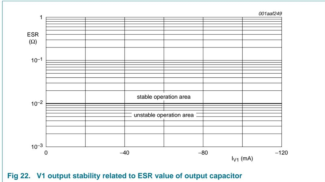
Fig 22. V1 output stability related to ESR value of output capacitor
