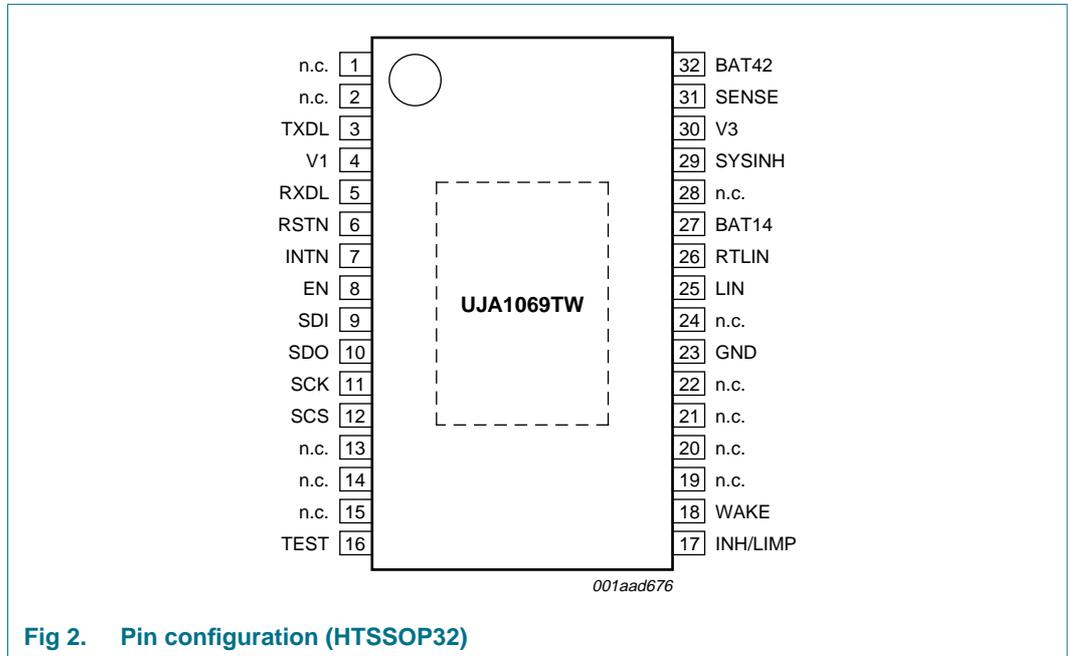
Fig 2. Pin configuration (HTSSOP32)
