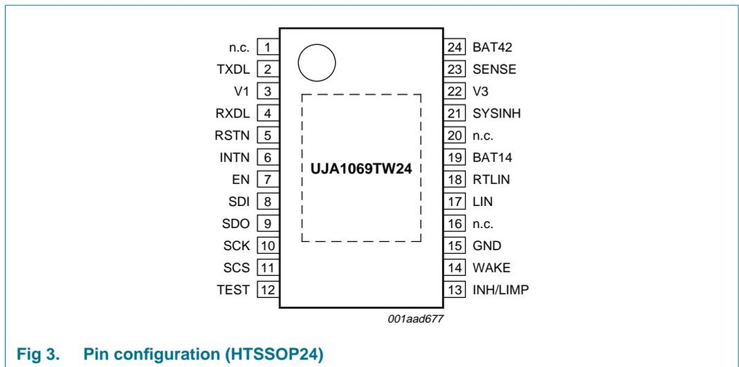
Fig 3. Pin configuration (HTSSOP24)
