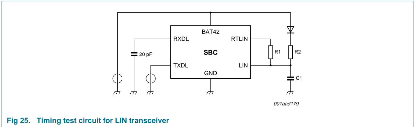
Fig 25. Timing test circuit for LIN transceiver
