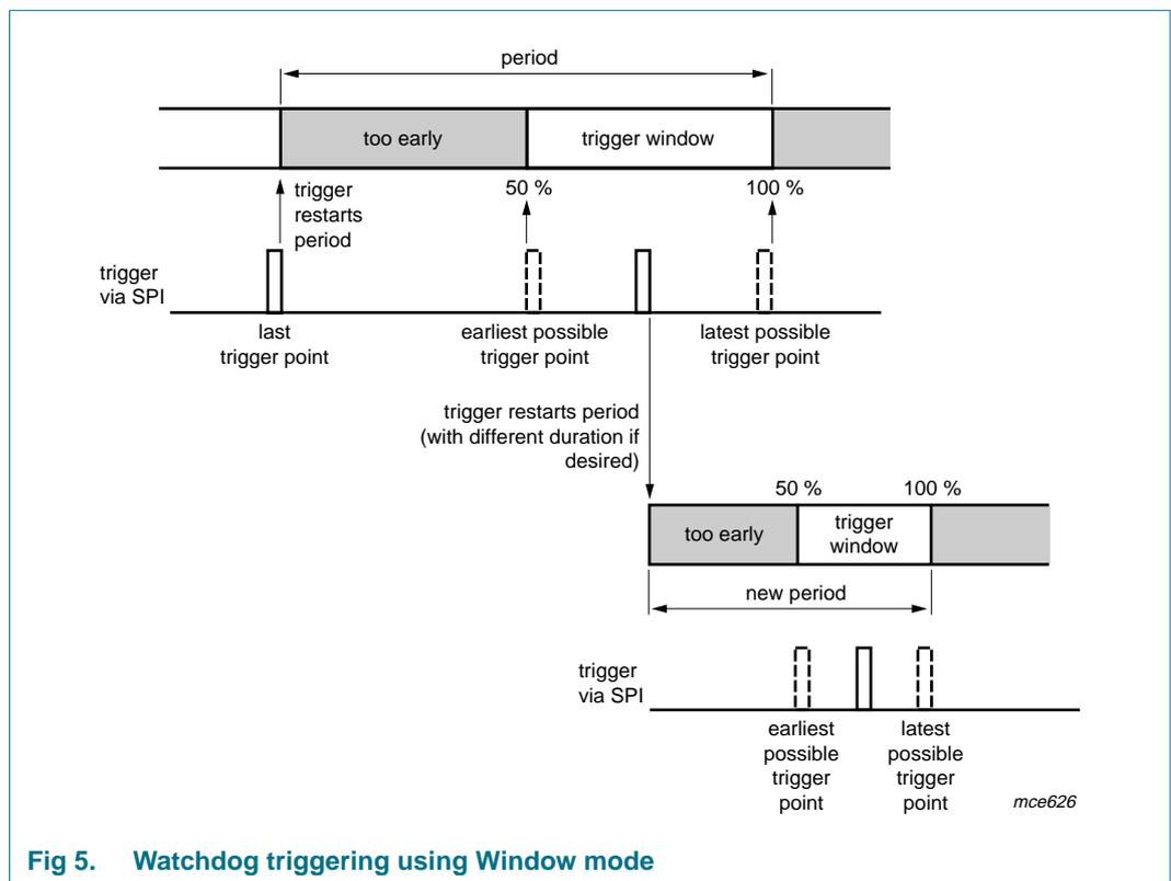
**Fig 5. Watchdog triggering using Window mode**
