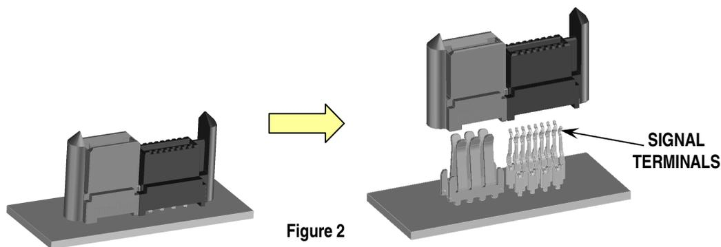
2. Use a needle-nose pliers to remove any signal terminals left in the PCB.
