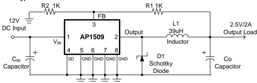
$$V_{OUT} = V_{FB} \times \left(1 + \frac{R1}{R2}\right)$$
