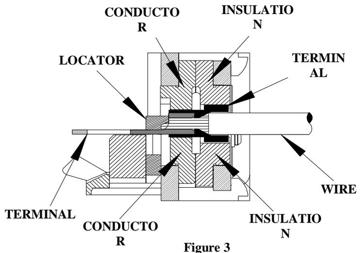
**Note:** Whenever crimping without the locator, make sure the seam of the terminal is oriented up or down in the tool if using unbrazed product, as this will provide higher pull force values.
