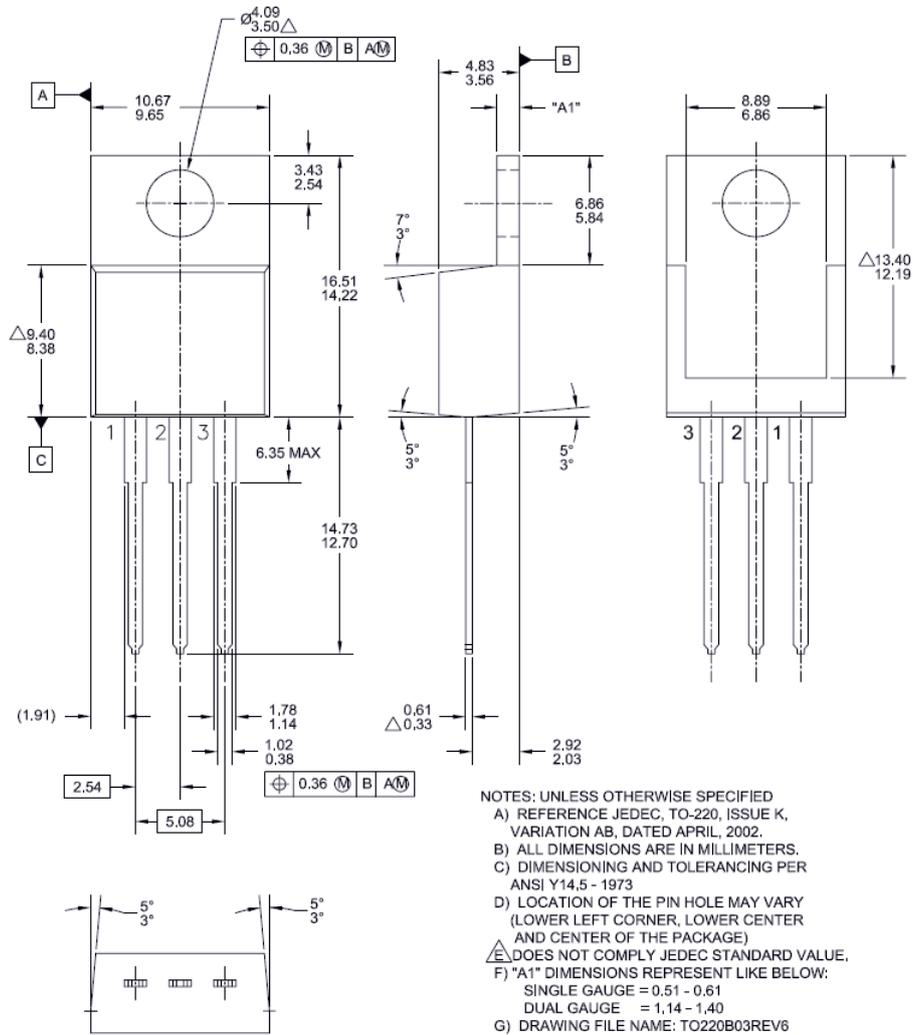
**Figure 20. TO-220 3L - TO-220, MOLDED, 3LEAD, JEDEC VARIATION AB**
