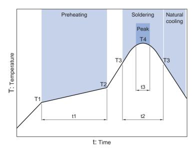
Preheating Soldering Peak Temp. Time Temp. Time Temp. Time T1 T2 Т3 **T4** 150°C 180°C 60 to 120s 230°C 250 to 260°C 30 to 60s 10s
