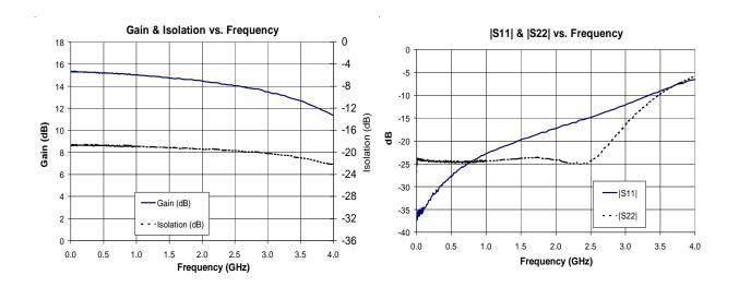
Typical RF Performance - Single Ended - 37.5 Ohm System  $V_s$ =8V,  $I_D$ =80mA (one amp biased),  $T_L$ =+25°C,  $R_{BIAS}$ =33 Ohms
