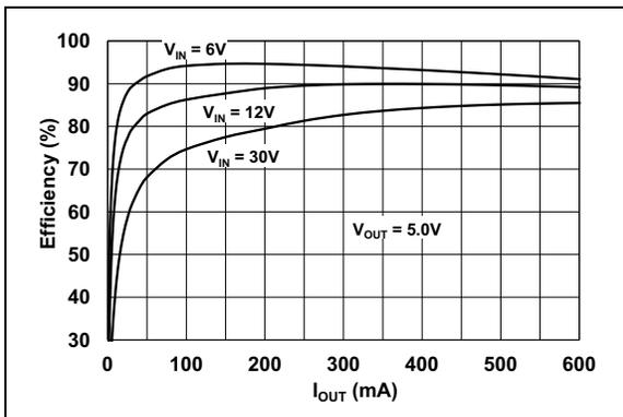
**FIGURE 2-3:** 5.0V  $V_{OUT}$  Efficiency vs.  $I_{OUT}$ .
