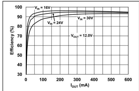
**FIGURE 2-4:** 12V  $V_{OUT}$  Efficiency vs.  $I_{OUT}$ .
