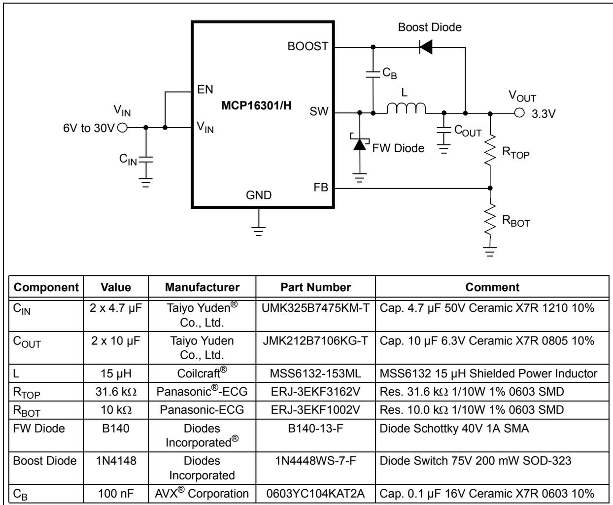
**FIGURE 6-1:** Typical Application 30V  $V_{IN}$  to 3.3V  $V_{OUT}$ .
