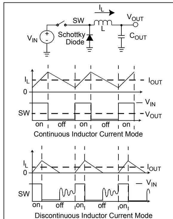
**FIGURE 4-2:** Step-Down Converter.
