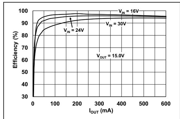
**FIGURE 2-5:** 15V  $V_{OUT}$  Efficiency vs.  $I_{OUT}$ .
