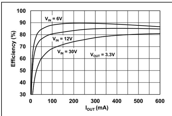
**FIGURE 2-2:** 3.3V  $V_{OUT}$  Efficiency vs.  $I_{OUT}$ .
