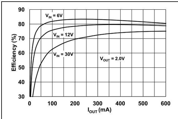
**FIGURE 2-1:** 2.0V  $V_{OUT}$  Efficiency vs.  $I_{OUT}$ .
