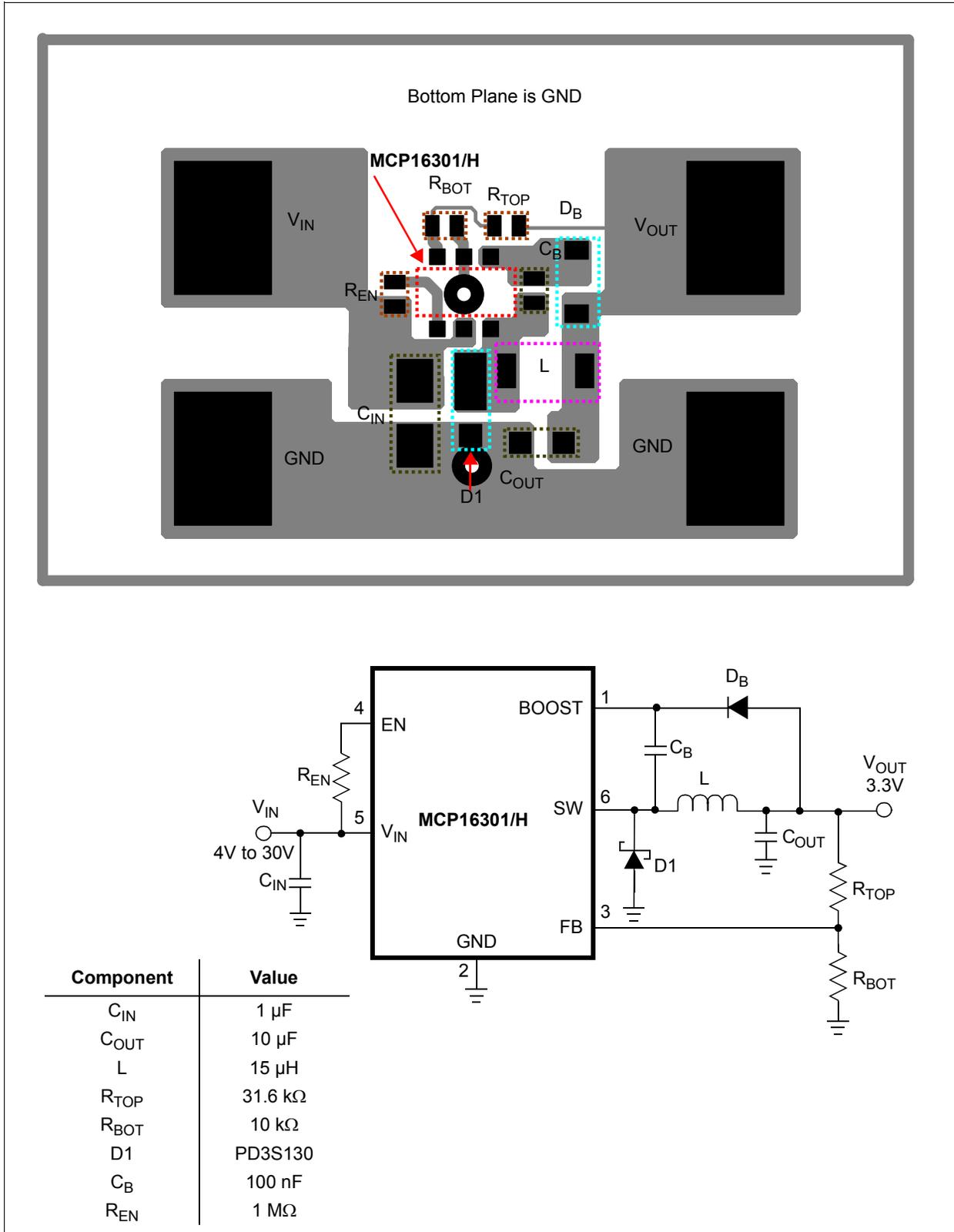
**FIGURE 5-2:** MCP16301/H SOT-23-6  $D^2$  Recommended Layout, 200 mA Design.
