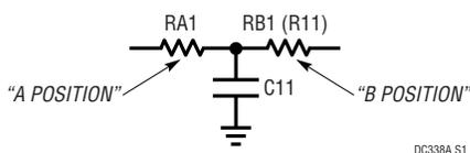
Note that the RB1 resistor is double labeled as RB1(R11). This is done to conform with the schematic that FilterCAD provides. If the section is 3rd order, using a TEE network, the two resistors are labeled as RA1 and RB1 (RA2 and RB2 for section B) by FilterCAD. If the section is a standard 2nd order, the one resistor is labeled R11 (R12 for section B) by FilterCAD.
