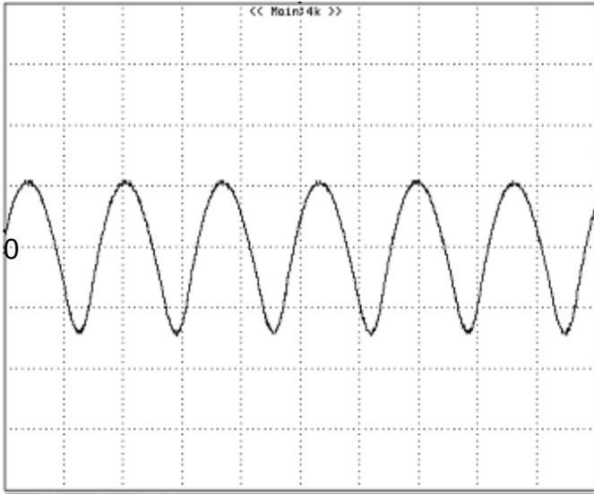
**Figure 11:** Input Terminal Ripple Current,  $i_c$ , at full rated output current and nominal input voltage with  $12\mu\text{H}$  source impedance and  $33\mu\text{F}$  electrolytic capacitor (500 mA/div, 2us/div).
