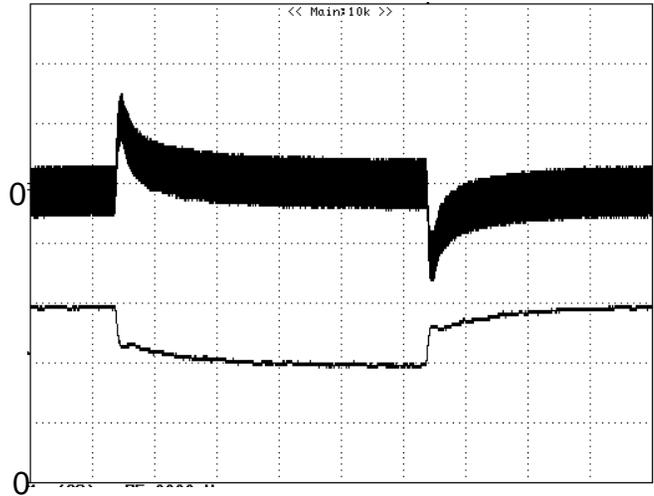
**Figure 9:** Output voltage response to step-change in load current (75%-50%-75% of  $I_{o, \max}$ ;  $di/dt = 1A/\mu s$ ). Load cap:  $330\mu F$ ,  $35m\Omega$  ESR solid electrolytic capacitor and  $1\mu F$  ceramic capacitor. Top Trace:  $V_{out}$  (100mV/div, 200us/div), Bottom Trace:  $I_{out}$  (3.75A/div). Scope measurement should be made using a BNC cable (length shorter than 20 inches). Position the load between 51 mm to 76 mm (2 inches to 3 inches) from the module.
