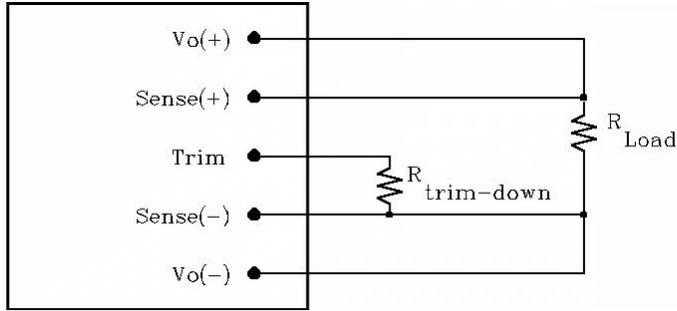
**Figure 18:** Circuit configuration for trim-down (decrease output voltage)
