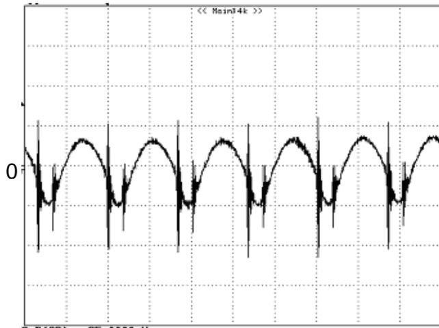
**Figure 14:** Output voltage ripple at nominal input voltage and rated load current ( $I_o=10A$ ) (10 mV/div, 2 us/div)
