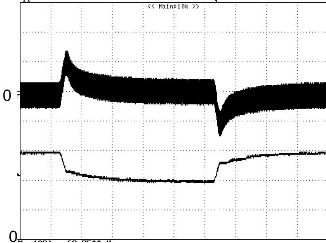
**Figure 8:** Output voltage response to step-change in load current (75%-50%-75% of  $I_{o, \max}$ ;  $di/dt = 0.1A/\mu s$ ). Load cap:  $10\mu F$ , tantalum capacitor and  $1\mu F$  ceramic capacitor. Top Trace:  $V_{out}$  (100mV/div, 200us/div), Bottom Trace:  $I_{out}$  (3.75A/div). Scope measurement should be made using a BNC cable (length shorter than 20 inches). Position the load between 51 mm to 76 mm (2 inches to 3 inches) from the module.
