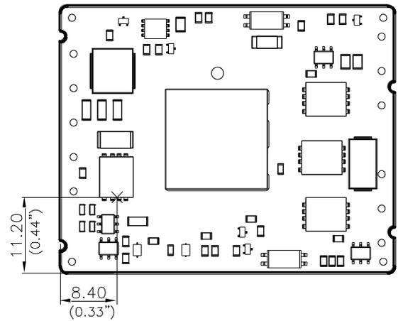
Figure 21: Temperature measurement location
