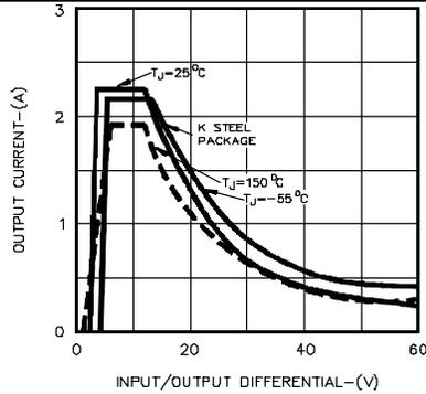
**Figure 2 – Output Current vs. Input / Output Differential**
