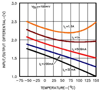
**Figure 4 – Input / Output Differential vs. Temperature**
