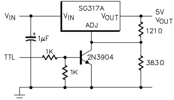
**Figure 22 – 5V Regulator with Shut Down**
