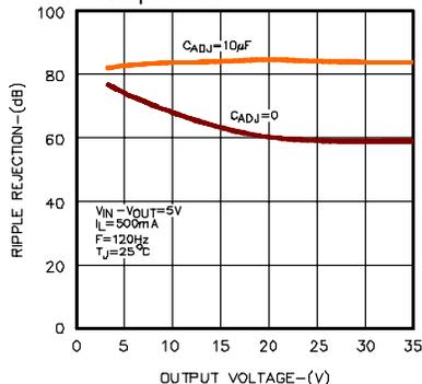
**Figure 7 – Ripple Rejection vs. Output Voltage**
