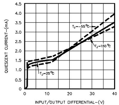
**Figure 6 – Quiescent Current vs. Input / Output Differential**
