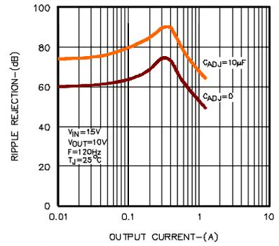
**Figure 9 – Ripple Rejection vs. Output Current**
