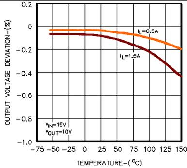
**Figure 1 – Output Voltage Deviation vs. Temperature**
