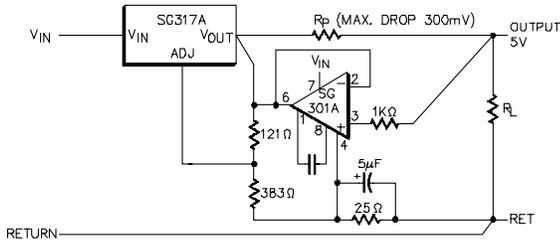
**Figure 20 – Remote Sensing**
