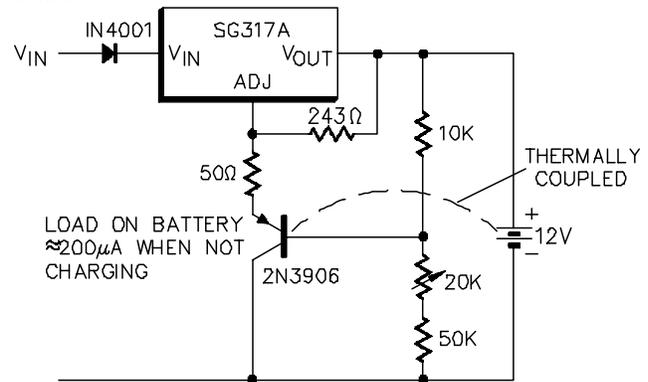
**Figure 25 – Temperature Compensated Lead Acid Battery Charger**
