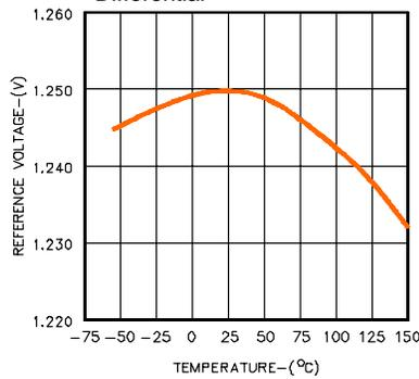
**Figure 5 – Reference Voltage vs. Temperature**
