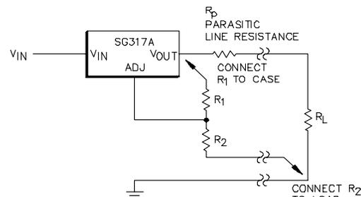
**Figure 18 – Connections for Best Load Regulation**
