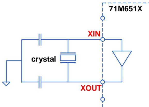
Figure 9: Oscillator Circuit
