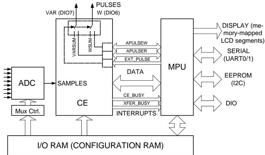
**Figure 18: MPU/CE Communication (Functional)**
