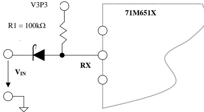
**Figure 36: Interfacing RX to a 0-5V Signal**
