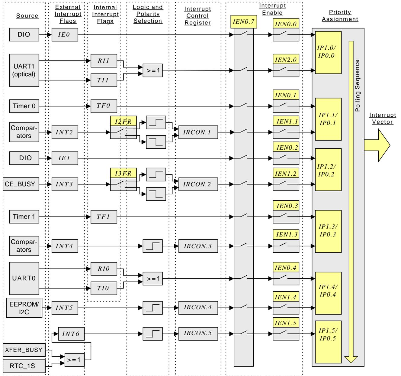
Figure 7: Interrupt Structure
