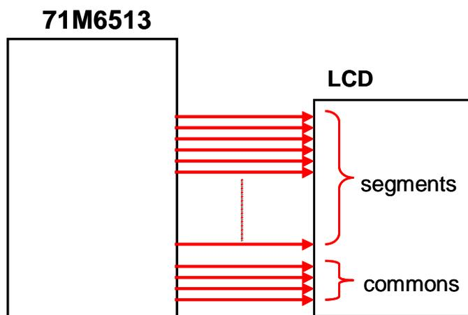
Figure 33: Connecting LCDs
