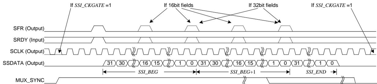
**Figure 15: SSI Timing, ( $SSI\_FPOL = SSI\_RDYPOL = 0$ )**
