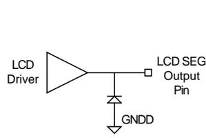
**LCD Output Equivalent Circuit**
