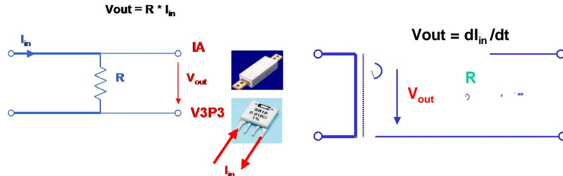
Figure 28: Resistive Shunt (left), Rogowski Coil (right)
