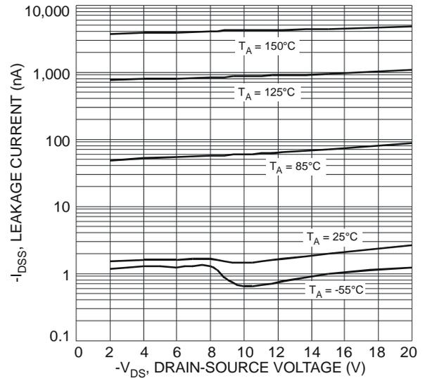
Figure 12 Typical Leakage Current vs. Drain-Source Voltage
