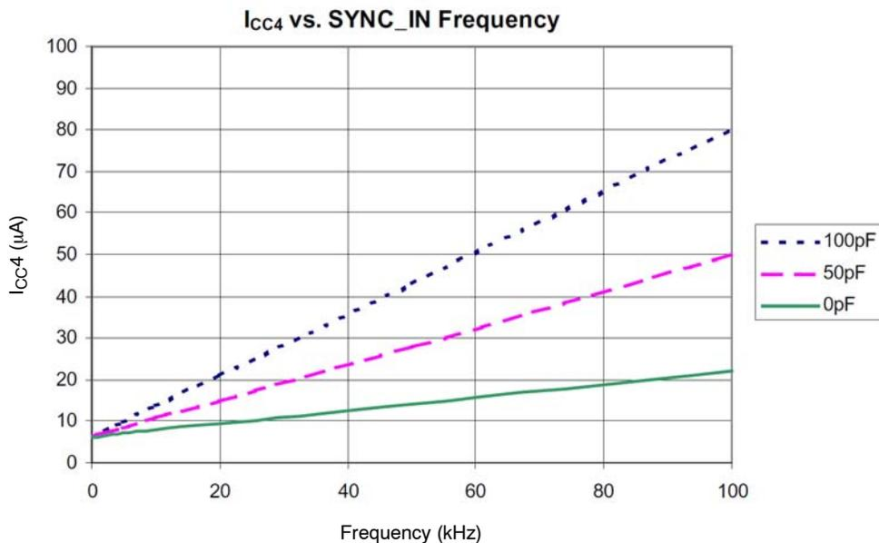
Figure 2.  $I_{CC4}$  vs. SYNC\_IN Frequency Performance Data
