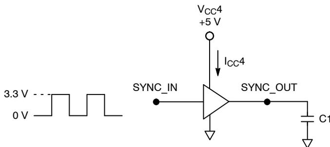
Figure 1. Sync Buffer  $I_{CC4}$  Test Circuit
