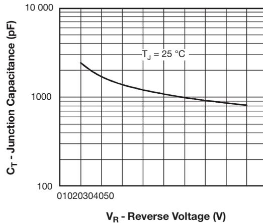
Fig. 1 - Typical Junction Capacitance vs. Reverse Voltage
