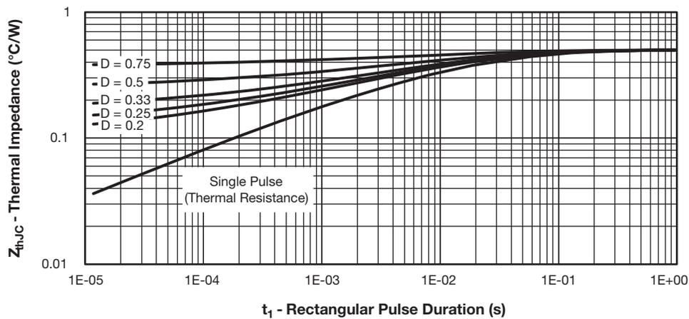
Fig. 3 - Maximum Thermal Impedance  $Z_{thJC}$  Characteristics
