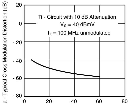
Fig. 3 - Typ. Cross Modulation Distortion vs. Frequency  $f_2$
