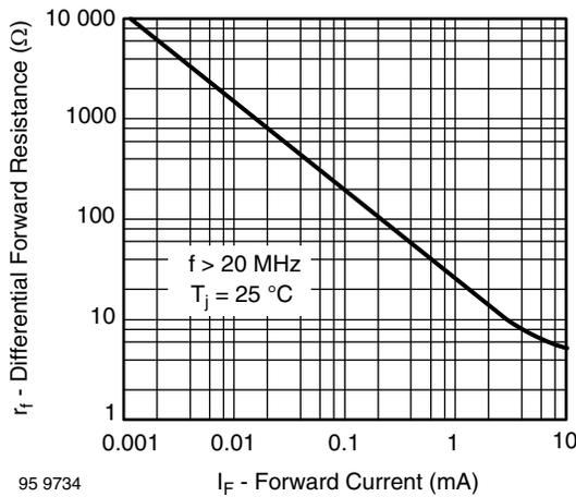
Fig. 2 - Differential Forward Resistance vs. Forward Current
