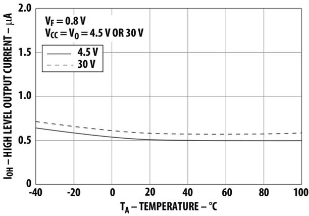
Figure 4. High Level Output Current vs. Temperature.
