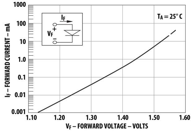
Figure 5. Input Current vs. Forward Voltage.
