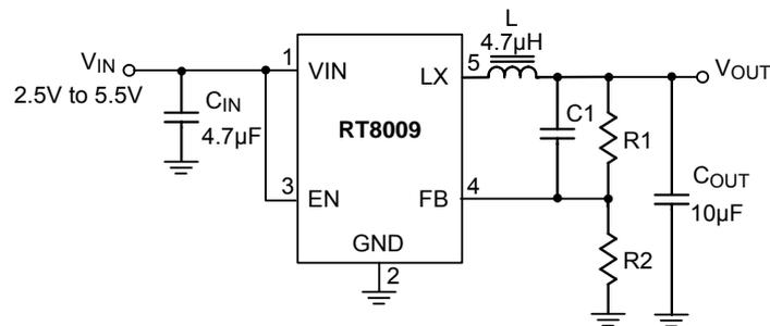
$$V_{OUT} = V_{REF} \times \left(1 + \frac{R1}{R2}\right)$$
