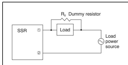
In case the dummy resistor is not used, keep in mind that the residual voltage becomes as follows:
