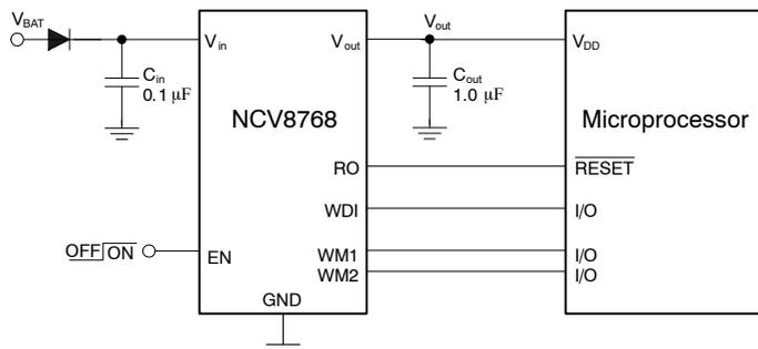
Figure 1. Application Schematic
