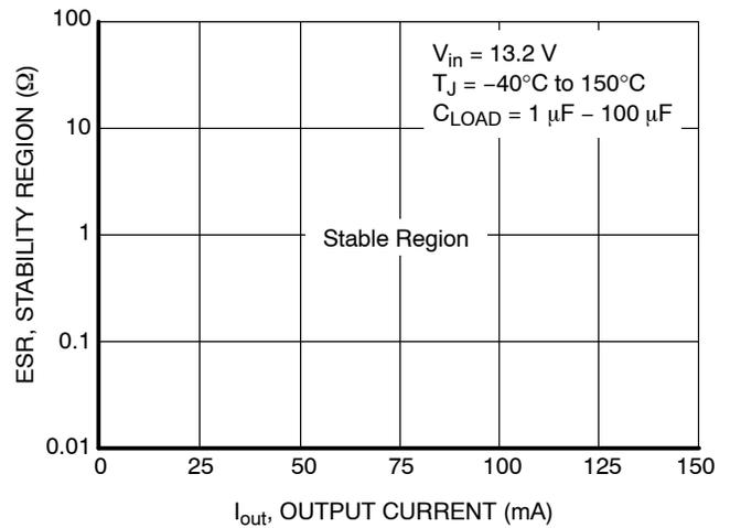
Figure 13.  $C_{out}$  ESR Stability Region vs Output Current
