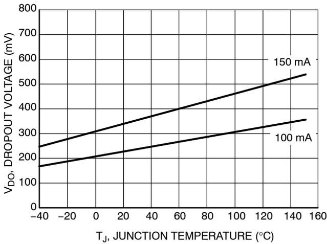
Figure 10. Dropout vs Temperature
