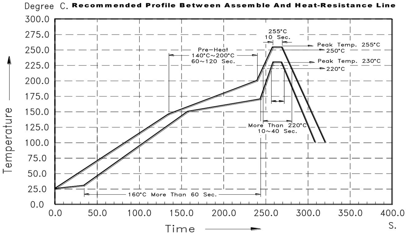
The Profile is available that must to use SnAg (x=3.3~3.8) Cu (y=0.2~0.7) solder paste
