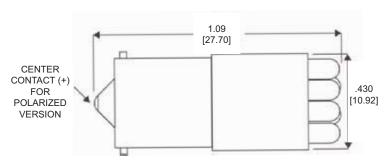
Measurements are typical Dimensions are inches [mm]
