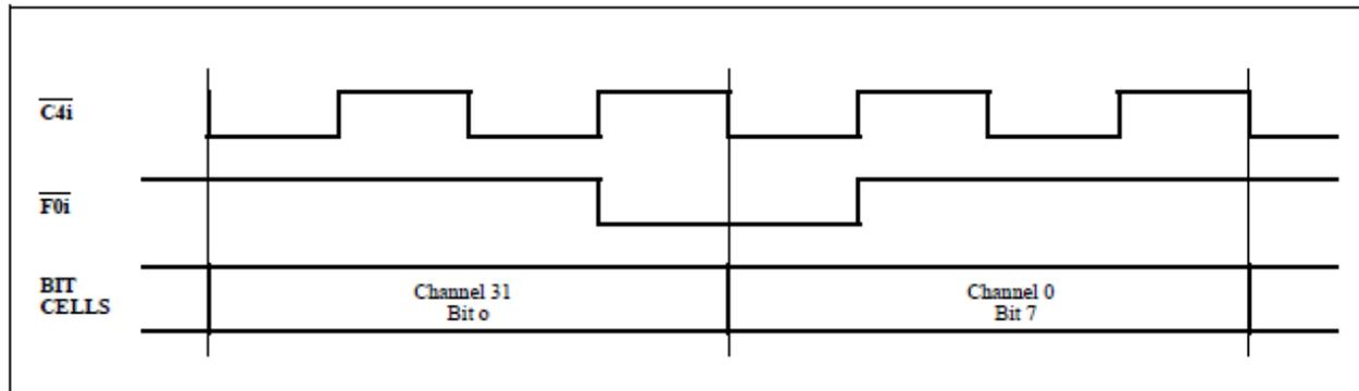
Figure 12 - Frame Alignment
