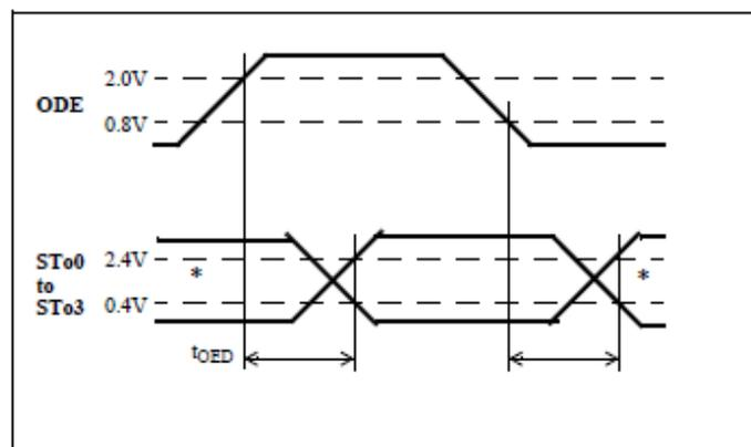
Figure 15 - Output Driver Enable
