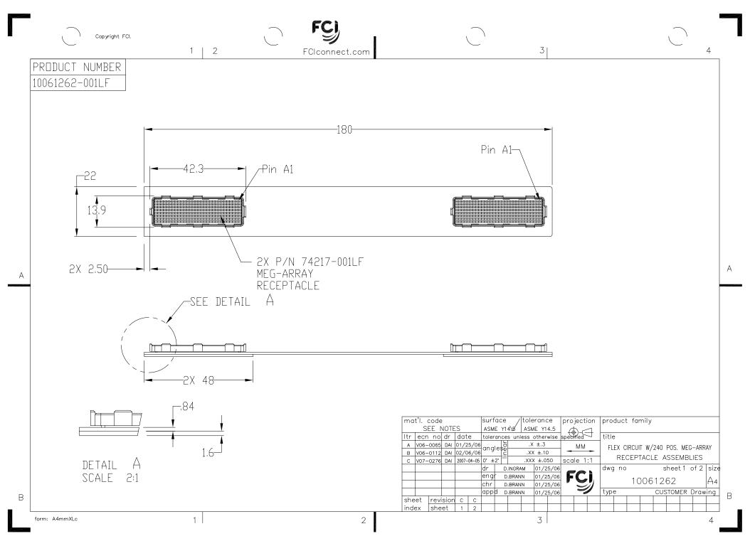
MM FLEX CIRCUIT W/240 POS. MEG-ARRAY .XX ±.10 RECEPTACLE ASSEMBLIES scale 1:1 0° ±2° .XXX ±.050 dwg no sheet2 of dr D.INGRAM 01/25/06 size D.BRANN 01/25/06 10061262 Α4 lchr D.BRANN 01/25/06 CUSTOMER Drawing appd D.BRANN 01/25/06 type sheet revision index sheet form: A4mmXLc 1 2 3
