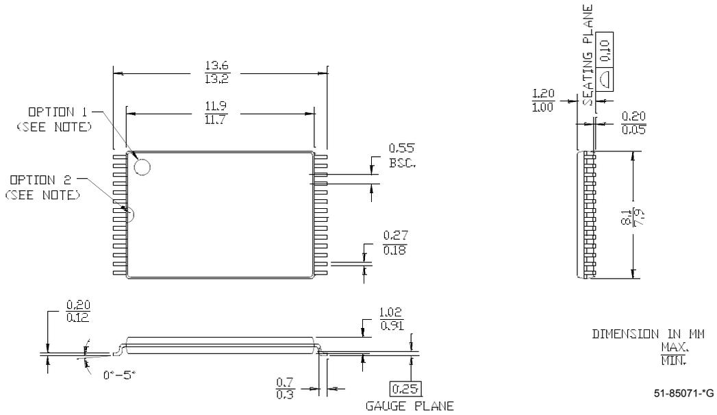
Figure 13. 28-Pin TSOP I (8 x 13.4 mm) (51-85074)
