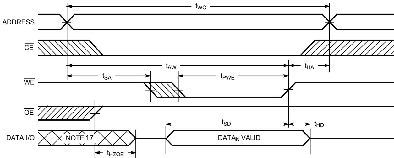
Figure 8. Write Cycle No. 2 ( $\overline{CE}$  Controlled)<sup>[10, 15, 16]</sup>
