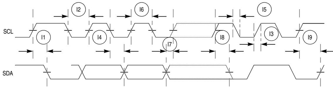
Figure 7. I<sup>2</sup>C Input/Output Timings
