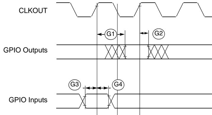
Figure 5. GPIO Timing
