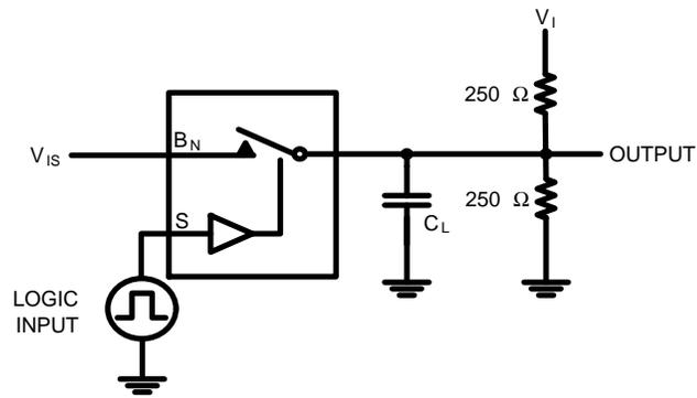
**Note:** Input  $V_{IS}$  driven by  $50\ \Omega$  source terminated by  $50\ \Omega$ .
