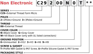
$\textbf{no digit} = \textbf{Single Bag Unmounted}, \ \textbf{SN} = \textbf{Bulk Pack Mounted}, \ \textbf{CN} = \textbf{Bulk Pack Unmounted}$
