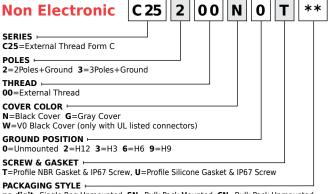
no digit=Single Bag Unmounted, SN=Bulk Pack Mounted, CN=Bulk Pack Unmounted
