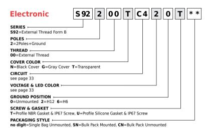
mPm® Field Attachable DIN Valve Connectors
