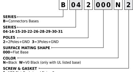
**Note:** UL listed part number identified by adding suffix SA at the end of the nomenclature in conjunction with UL material (W for black and T for transparent) e.g. B142000W2SA
