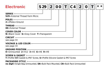
**Note:** UL listed part number identified by adding suffix SA at the end of the nomenclature in conjunction with UL material (W for black and T for transparent) e.g. C28200W2RSNSA
