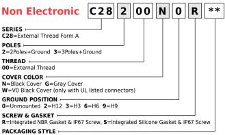
$\textbf{no digit} = \textbf{Single Bag Unmounted}, \ \textbf{SN} = \textbf{Bulk Pack Mounted}, \ \textbf{CN} = \textbf{Bulk Pack Unmounted}$
