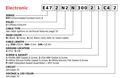
**Note:** UL listed part number identified by combining UL listed cable with UL overmolding material e.g. E152A3A30011
