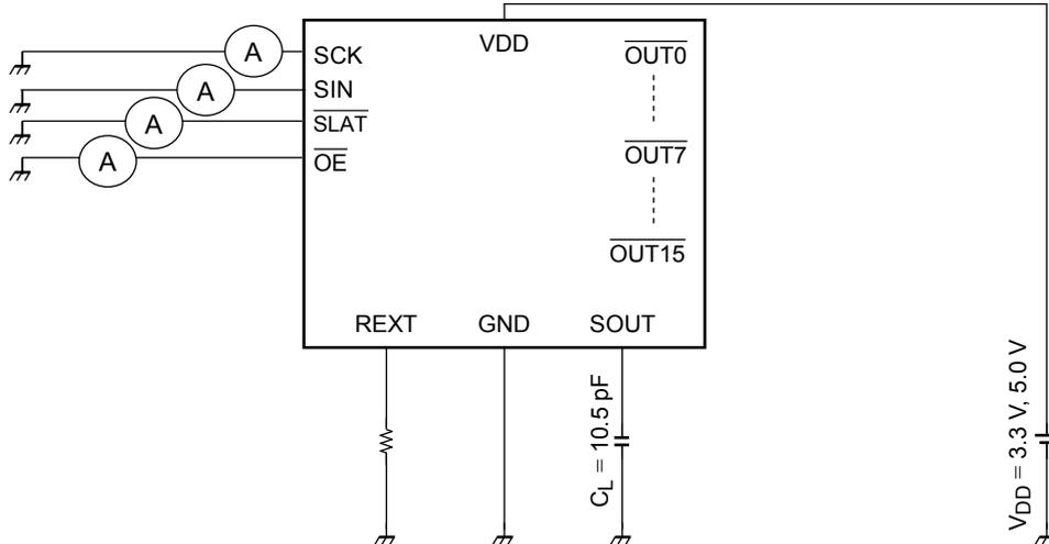
Test Circuit4: Power supply current
