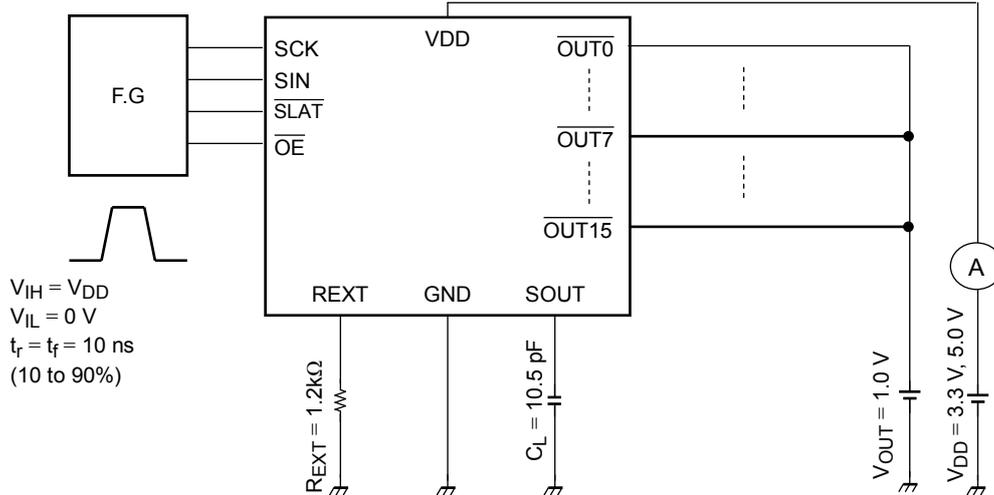
Test Circuit5: Constant current output / Output OFF leak current / Constant current error
