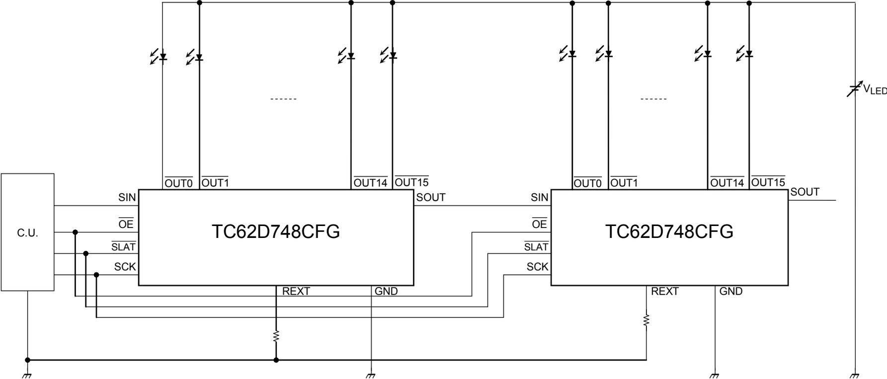
Application Circuit: General Composition for Dynamic Lighting of LEDs
