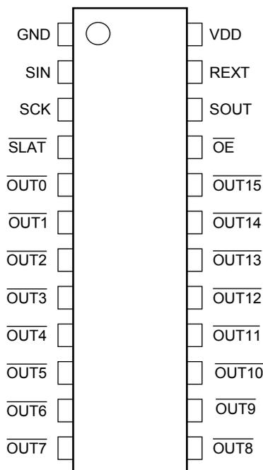
Short circuiting an output pin to a power supply pin (Power-supply voltage  $V_{DD}$  and LED anode power supply), or short-circuiting the REXT pin to the GND pin will likely exceed the absolute maximum rating, which in turn may result in smoldering and/or permanent damage. Please keep this in mind when determining the wiring layout for the power supply and GND pins.
