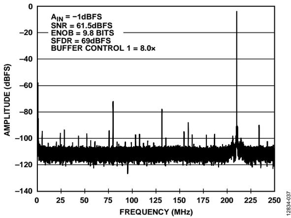
Figure 37. Single-Tone FFT with  $f_{IN} = 1710.3$  MHz
