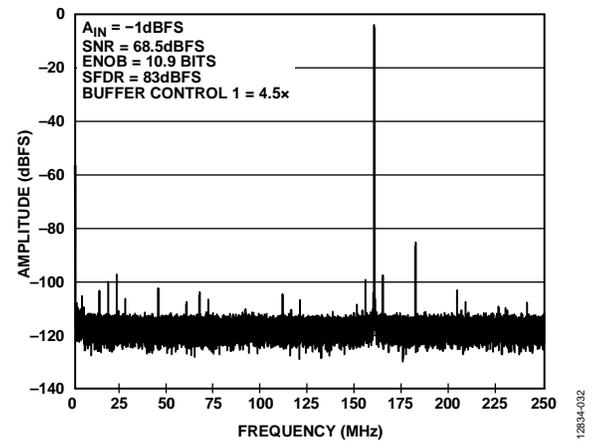
Figure 32. Single-Tone FFT with  $f_{IN} = 340.3$  MHz
