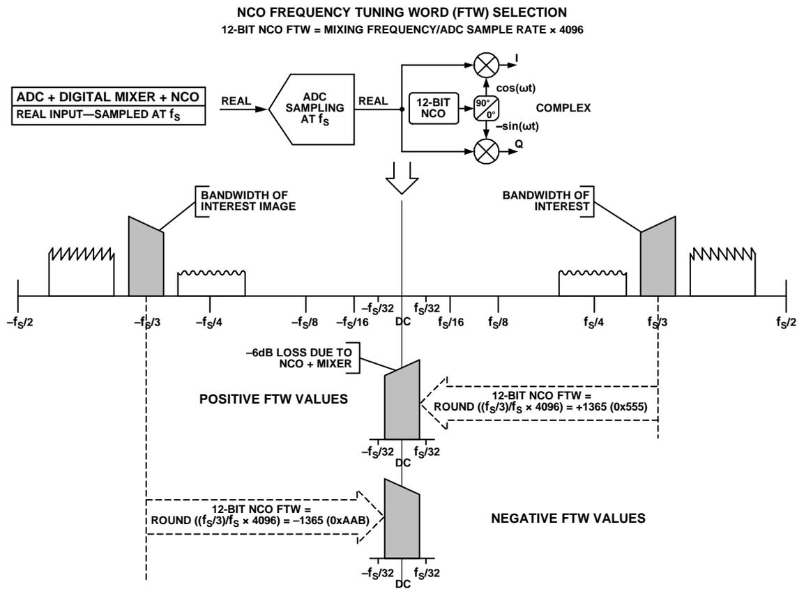
Figure 90. DDC NCO Frequency Tuning Word Selection—Real Inputs
