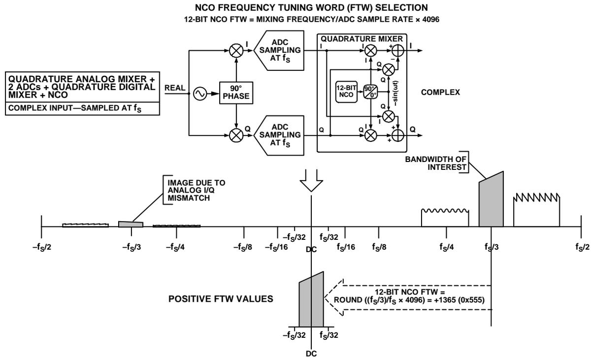
Figure 91. DDC NCO Frequency Tuning Word Selection—Complex Inputs
