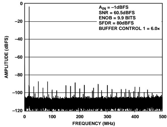
Figure 11. Single-Tone FFT with  $f_{IN} = 985.3$  MHz
