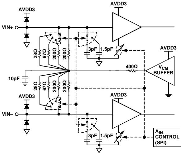
Figure 53. Analog Inputs
