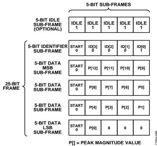
Figure 86. SPORT over JESD204B Signal Monitor Frame Data
