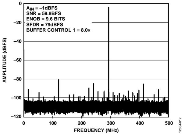
Figure 12. Single-Tone FFT with  $f_{IN} = 1293.3$  MHz
