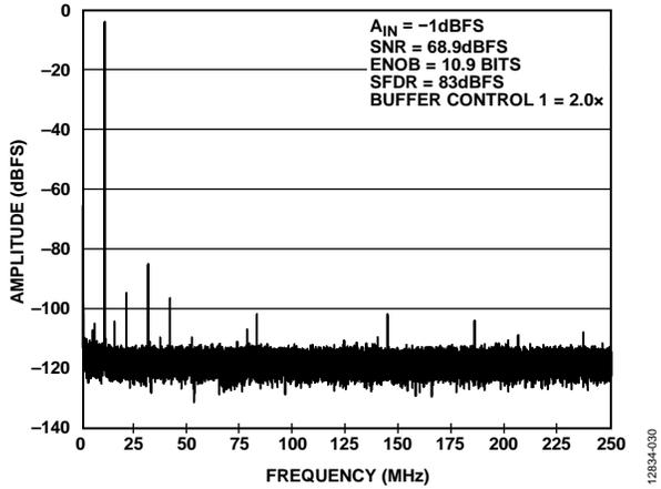
Figure 30. Single-Tone FFT with  $f_{IN} = 10.3$  MHz
