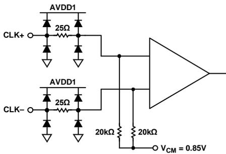
Figure 54. Clock Inputs
