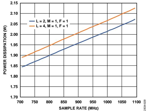
Figure 29. Power Dissipation vs. Sample Rate ( $f_s$ )
