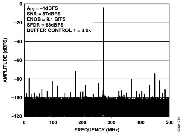
Figure 14. Single-Tone FFT with  $f_{IN} = 1950.3$  MHz
