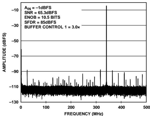
Figure 8. Single-Tone FFT with  $f_{IN} = 340.3$  MHz
