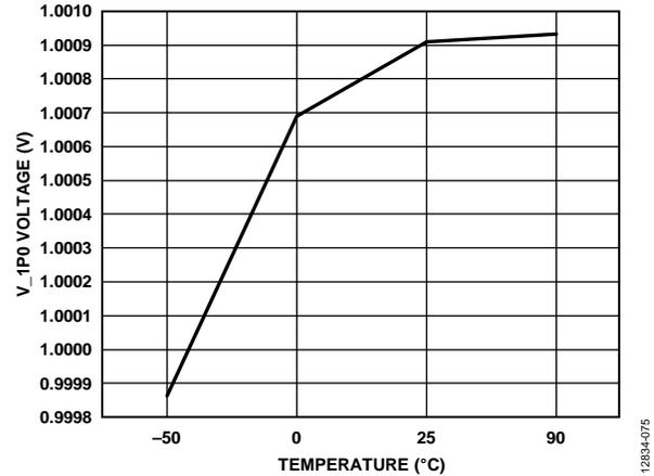
Figure 75. Typical V<sub>1P0</sub> Drift
