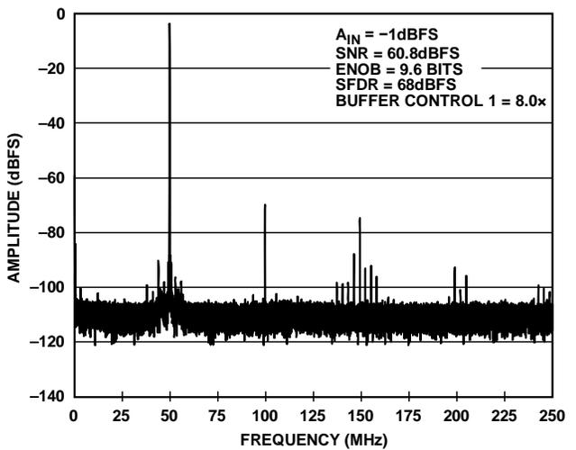
Figure 38. Single-Tone FFT with  $f_{IN} = 1950.3$  MHz
