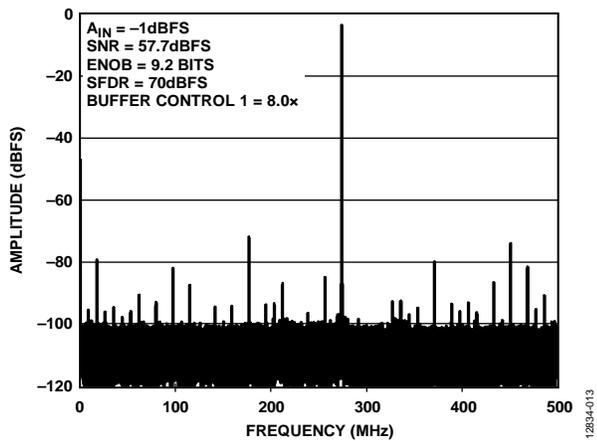
Figure 13. Single-Tone FFT with  $f_{IN} = 1725.3$  MHz
