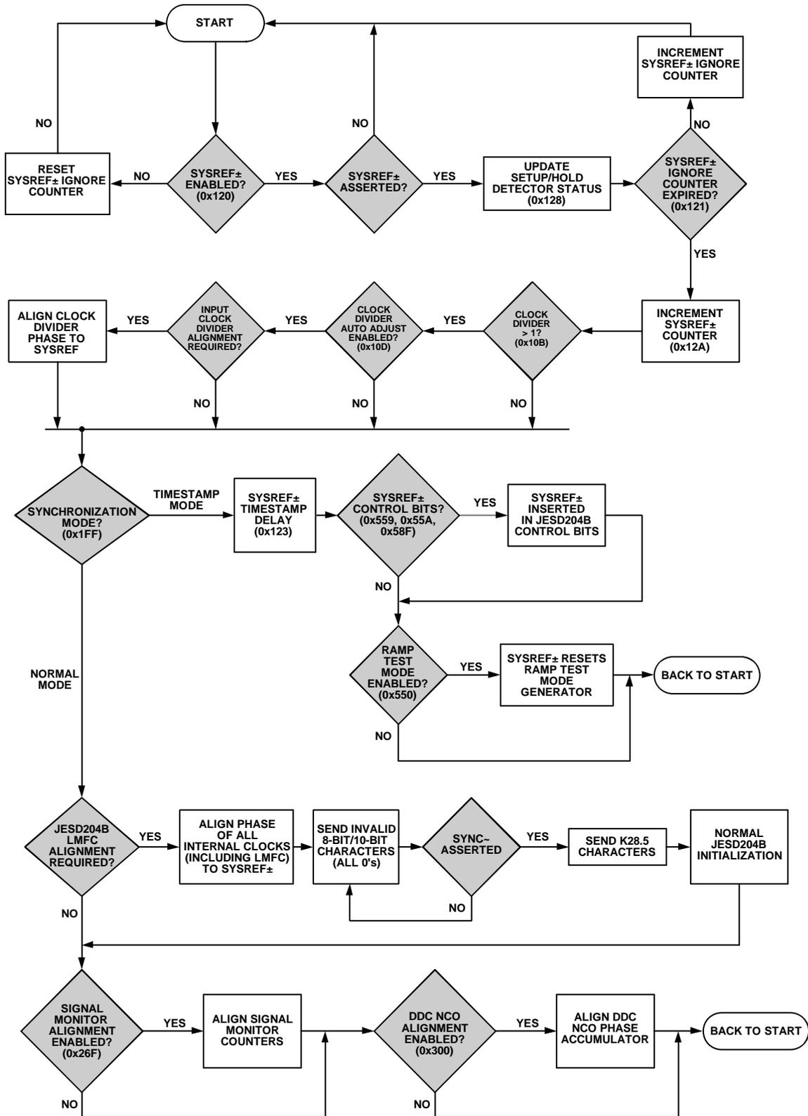
Figure 111. Multichip Synchronization
