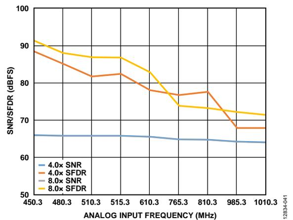
Figure 41. SNR/SFDR vs.  $f_{IN}$ ;  $500$  MHz  $< f_{IN} < 1$  GHz; Buffer Control 1 (0x018) = 4.0x and 8.0x
