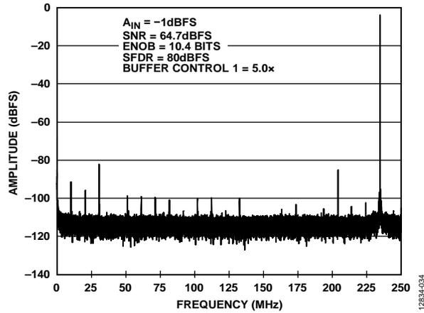
Figure 34. Single-Tone FFT with  $f_{IN} = 765.3$  MHz
