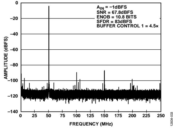
Figure 33. Single-Tone FFT with  $f_{IN} = 450.3$  MHz
