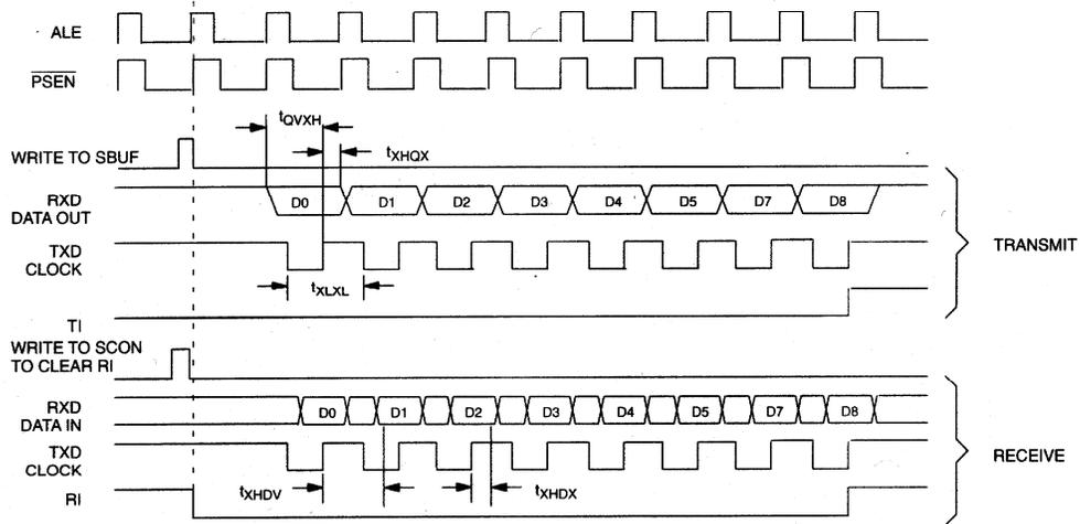
SERIAL PORT 0 (SYNCHRONOUS MODE)
