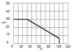
Maximum Forward DC Current vs. Ambient Temperature
