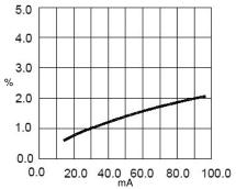
Relative Luminous Flux vs. Forward Current
